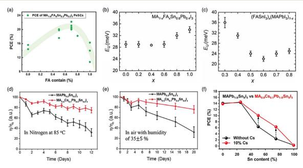
Fig. 10 (a) PCE of  $MA_{1-x}FA_xSn_{0.5}Pb_{0.5}I_3$  PSCs. UE in relation to the changing perovskite composition for (b)  $MA_{1-x}FA_xPb_{0.4}Sn_{0.6}I_3$  and (c)  $(FASnI_3)_x(MAPbI_3)_{1-x}$ . (d-f) Thermal and air stability test conducted on the device at 85 °C with 10% Cs addition. Stability and efficiency increase with the inclusion of Cs in  $Sn_xPb_{1-x}$  PSCs. (b and c) Ref. 143. (d-f) Ref. 144.
