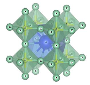
Fig. 2 ABX<sub>3</sub> crustal of perovskite materials.
