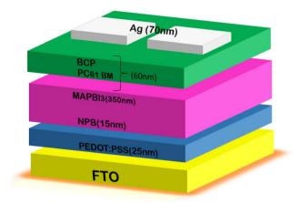
Fig. 14 Structure of the PSC based on NPB.
