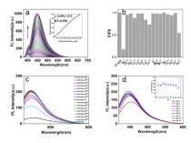
Fig. 6 (a) PL spectra of aqueous GF-CD solutions at different concentrations excited at 400 nm. (Inset) peak PL intensity as a function of GF-CD concentration. (b) PL intensity of the GF-CD solution in the presence of inorganic ions (1 mmol  $L^{-1}$ ). (c) PL spectra of GF-CD interaction with metal ions. (d) PL spectra within the pH range 3–11. (Inset) PL intensity within the pH range 3–11.
