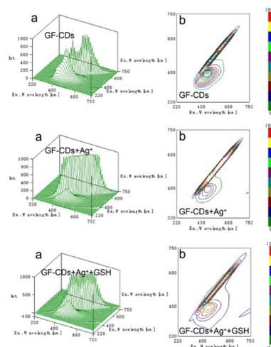
Fig. 10 (a) Three-dimensional PL spectra and (b) excitation–emission matrix (EEM) fluorescence spectra of GF-CDs-Ag<sup>+</sup>-GSH.
