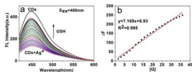
Fig. 11 (a) Fluorescence spectra of the GF-CDs-Ag<sup>+</sup>-GSH system at different GSH concentrations. (b) Linear relationship between  $\Delta F$  and GSH concentration.
