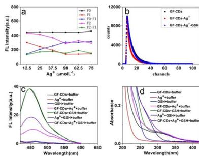
Fig. 9 (a) Effect of the Ag<sup>+</sup> concentration on the PL intensity of the GF-CD-Ag<sup>+</sup>-GSH system. (b) Fluorescence decay curve of the aqueous GF-CD-Ag<sup>+</sup>-GSH system solution. (c) Fluorescence spectra and (d) UV-vis absorption spectra of the GF-CD-Ag<sup>+</sup>-GSH system.
