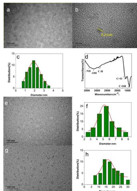
Fig. 3 (a) TEM image of GF-CDs. (b) HRTEM image of GF-CDs. (c) Associated particle size distribution of GF-CDs. (d) FTIR spectra of GF-CDs. (e) TEM image of GF-CDs- $\text{Ag}^+$ . (f) Associated particle size distribution of GF-CDs- $\text{Ag}^+$ . (g) TEM image of GF-CDs- $\text{Ag}^+$ -GSH. (h) Associated particle size distribution of GF-CDs- $\text{Ag}^+$ -GSH.
