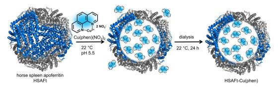
Fig. 1 Encapsulation of copper phenanthroline within HSAFt by the nanoreactor route. The removal of the iron core from ferritin yielded the empty HSAFt, which was loaded with the copper complex. The encapsulation by diffusion was performed by incubating the protein with an excess of the complex for 3 h at room temperature and pH 5.5. The sample was then dialysed to ensure the complete removal of residual unencapsulated compound.
