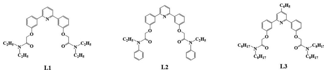
Fig. 2 Structure of phenylpyridine diamide extractants L1–L3.
