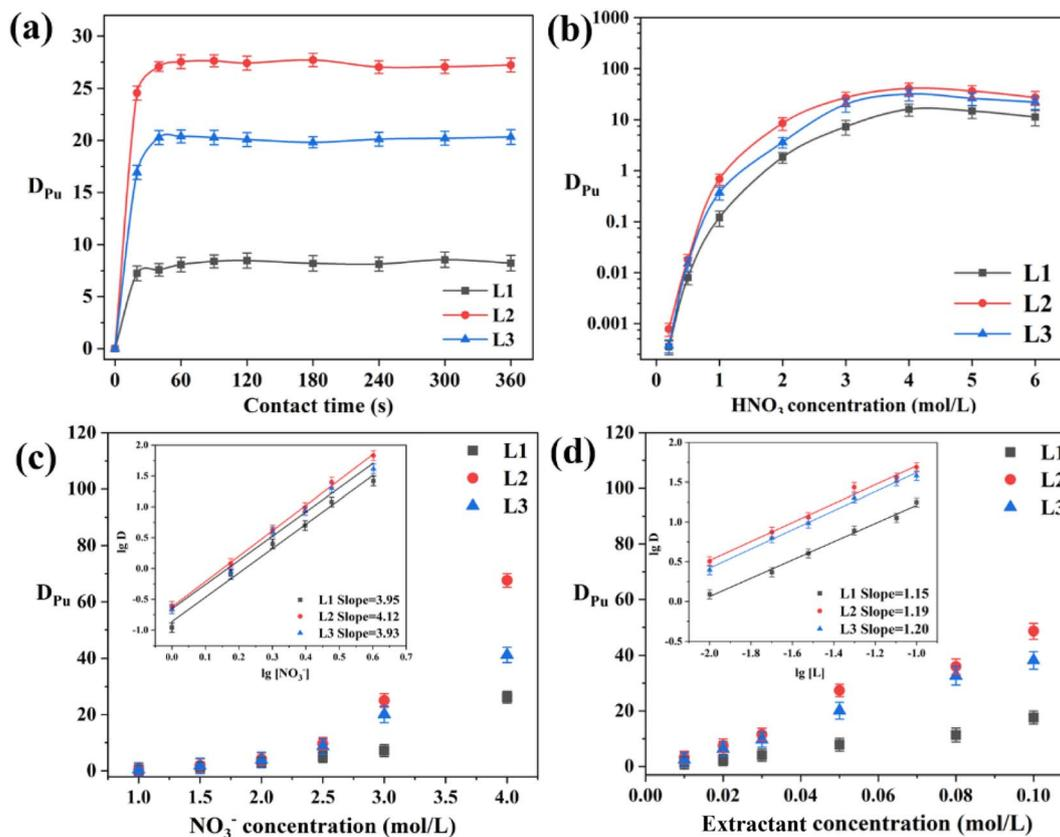
Fig. 3 (a) Kinetics of Pu(IV) extraction by phenylpyridine diamide ligands L1, L2, and L3. (b) Pu(IV) distribution ratios ( $D_{Pu}$ ) obtained for extractants at different  $HNO_3$  concentrations. (c) Influence of  $NO_3^-$  concentration on extraction performance. (d) Effect of extractant concentration on extraction performances of L1, L2, and L3.
