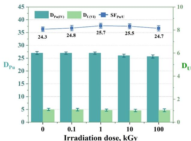
**Fig. 8** Extraction of Pu(IV) and U(VI) using L2 (PEPA) exposed to  $\gamma$  irradiation for different durations. Organic phase: 0.05 M L2 in 1-(trifluoromethyl)-3-nitrobenzene; aqueous phase: 3 M  $\text{HNO}_3$ , 5  $\text{mg L}^{-1}$  Pu(IV), and 1  $\text{g L}^{-1}$  U(VI).
