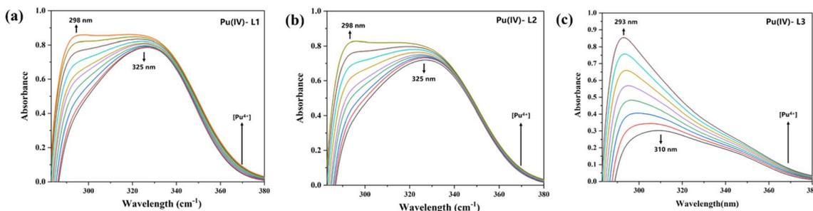
Fig. 5 Spectrophotometric titration of ligands (a) L1, (b) L2, and (c) L3 ([L] =  $2.0 \times 10^{-5}$  M) with Pu(NO<sub>3</sub>)<sub>4</sub> ([M] =  $2 \times 10^{-3}$  M) at  $T = 298$  K.
