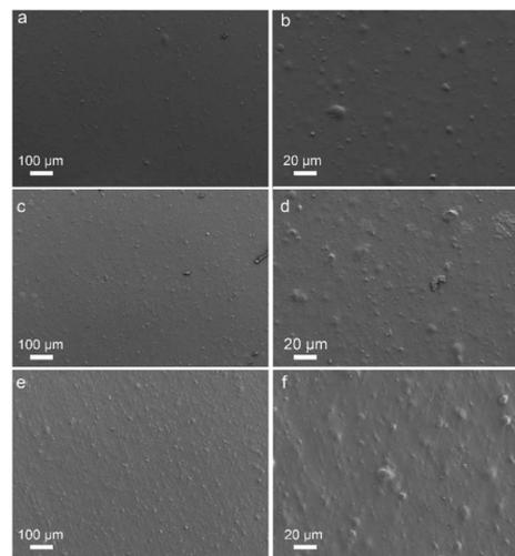
Fig. 2 SEM images of films (a and b) pure PBAT, (c and d) g-C<sub>3</sub>N<sub>4</sub> (0.25)/PBAT, and (e and f) g-C<sub>3</sub>N<sub>4</sub> (0.5)/PBAT.
