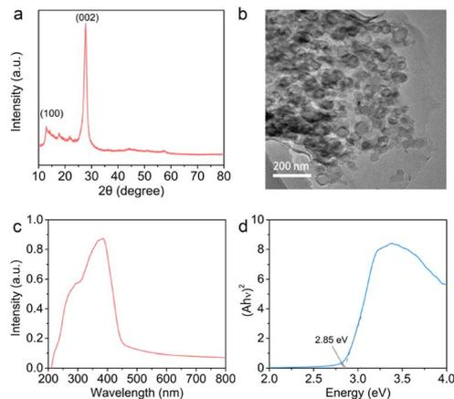
Fig. 1 (a) XRD patterns, (b) TEM image, (c) UV-Vis diffuse reflectance spectra, and (d) the corresponding Tauc plot of the prepared g-C<sub>3</sub>N<sub>4</sub>.
