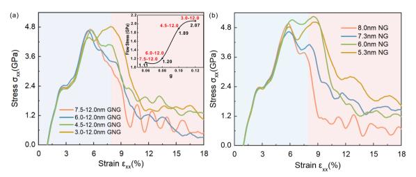
Fig. 2 Stress-strain curves for each model during tension (a) GNG model with different grain size gradients and (b) uniform NG model.
