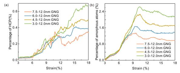
Fig. 10 Variation of the percentage of (a) HCP atoms and (b) amorphous atoms in the GNG model with different grain size gradients.
