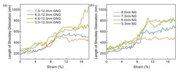
Fig. 9 Variation curves of the length of the Shockley dislocation during crack propagation for the GNG model and the NG model (a) GNG model (b) NG model.
