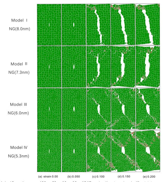
Fig. 4 (a-e) Propagation process of 8.0 nm, 7.3 nm, 6.0 nm, 5.3 nm NG MD samples with center cracks under different strains.
