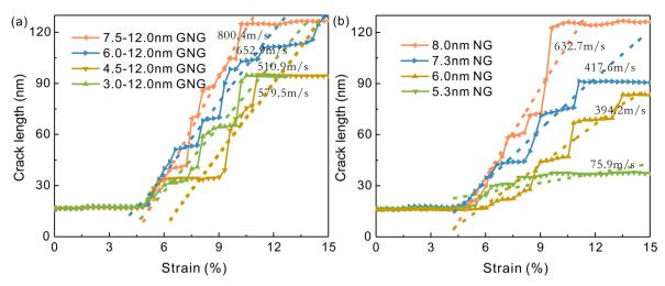
Fig. 5 Variation curve of crack length during crack propagation (a) GNG model (b) NG model.
