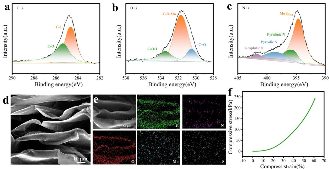
Fig. 4 (a) C 1s, (b) O 1s, and (c) N 1s XPS spectra of MoS<sub>2</sub>/C composites; (d) SEM images of MCA showing a vertical channel structure; (e) EDS mappings images of Mo, S, C, N, and O elements in MCA; (f) strain–stress curve of the compressive test of MCA.
