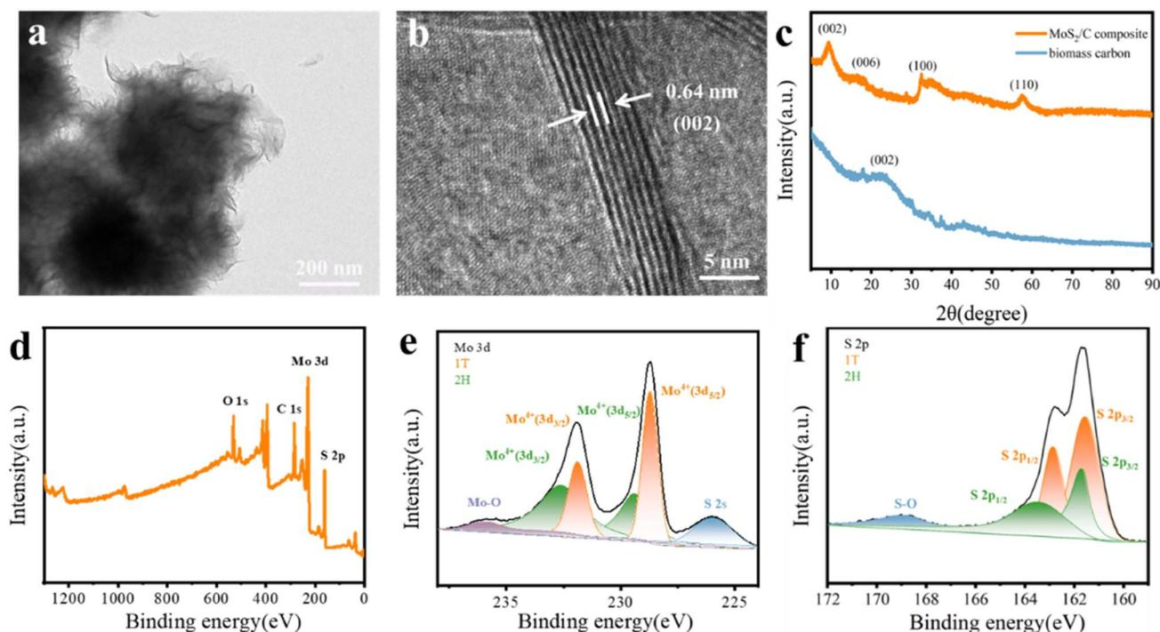
Fig. 3 (a) and (b) TEM and HRTEM images of  $\text{MoS}_2/\text{C}$  composites; (c) XRD patterns of the coconut shell-based biomass carbon and  $\text{MoS}_2/\text{C}$  composites; (d) survey XPS spectrum of  $\text{MoS}_2/\text{C}$  composites; (e) Mo 3d, and (f) S 2p XPS spectra of  $\text{MoS}_2/\text{C}$  composites.
