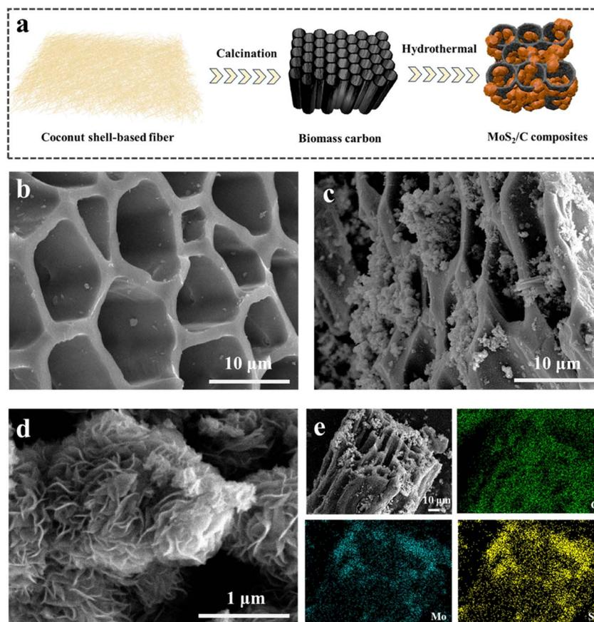
Fig. 2 (a) Schematic illustration for preparing  $\text{MoS}_2/\text{C}$  composites for Cu(II) ion removal; SEM images of (b) coconut shell-based biomass carbon and (c) and (d)  $\text{MoS}_2/\text{C}$  composites; (e) elemental mapping images of Mo, S, and C in  $\text{MoS}_2/\text{C}$  composites.
