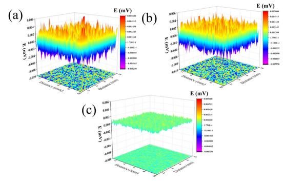
Fig. 3 Q235 in a 0.5 M  $H_2SO_4$  solution with and without 200 mg  $L^{-1}$  MXene inhibitor after different immersion times: 0 h (a, initial state), 24 h (b, without inhibitor), and 24 h (c, with inhibitor).
