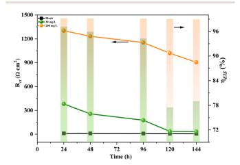
Fig. 2 Change of  $R_{\rm ct}$  and  $\eta_{\rm EIS}$  for Q235 carbon steel after immersion in 0.5 M H<sub>2</sub>SO<sub>4</sub> solution with varying concentrations (0, 30, and 200 mg L<sup>-1</sup>) of MXene.
