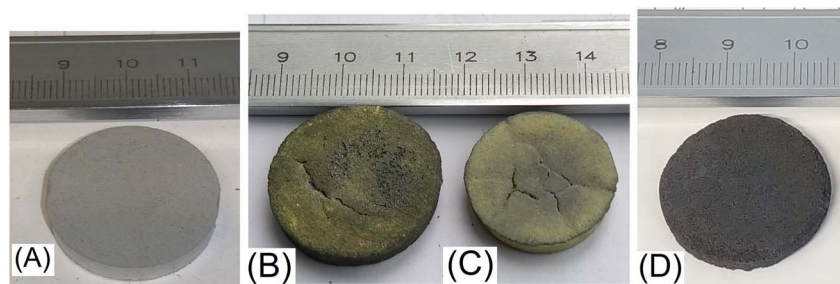
Fig. 1 Photographic images of the samples: Mo6 after pressing (A), Mo5 after sintering (B), Mo6 after sintering (C), Mo6 after sintering and etching in 10 M NaOH (D).
