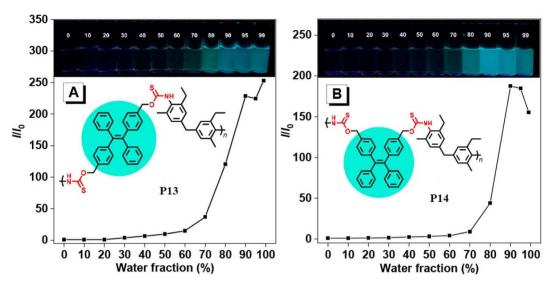
Fig. 2 Plots of relative PL intensity *versus* water fractions (by volume) in THF/water mixtures of (A) **P13** and (B) **P14**. Concentration of polymers:  $10 \mu$ M. Excitation wavelength:  $360 \mu$ M. This figure has been adapted/reproduced from ref.  $69 \mu$ M with permission from American Chemical Society, copyright 2021.
