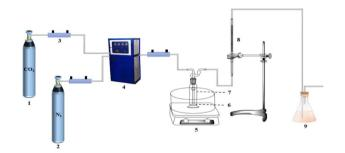
Fig. 3 Simulated flue gas experimental setup. (1)  $CO_2$  cylinder (2)  $N_2$  cylinder (3) rotor flow meter (4) gas mixer (5) collector type constant temperature magnetic stirrer (6) magneton (7) gas absorption cylinder (8) soap bubble flow meter (9) tail gas treatment device.
