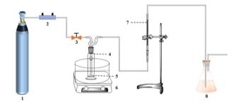
Fig. 1 Experimental setup for  $CO_2$  absorption. (1)  $CO_2$  cylinder (2) rotor flow meters (3) valve (4) gas absorption bottle (5) magneton (6) collector-type thermostatic magnetic stirrer (7) soap bubble flow meter (8) tail gas treatment unit.
