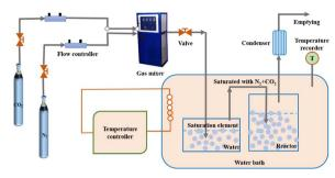
Fig. 5 Schematic diagram for the measurement of  ${\rm CO_2}$  equilibrium solubility.
