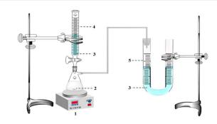
Fig. 4 Depleted-CO<sub>2</sub>-rich phase CO<sub>2</sub> loading measurement device. (1) magnetic stirrer (2) magnets (3) dilute hydrochloric acid (4) acid burette (5) U-tube.
