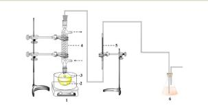
Fig. 2  $CO_2$  desorption device diagram. (1) Oil bath (2) magneton (3) single mouth flasks (4) snake condenser tube (5) soap bubble flow meter (6) tail gas treatment unit.
