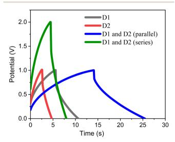
Fig. 8 GCD curves recorded for two different symmetric coin cell supercapacitor devices (D1 and D2) connected in parallel and series at a current density of 1 mA  $\rm cm^{-2}$ .
