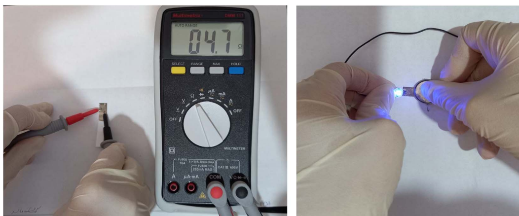
Fig. 1 Photographic image of conductivity and resistance of photographic paper impregnated with conductive silver nano-ink.
