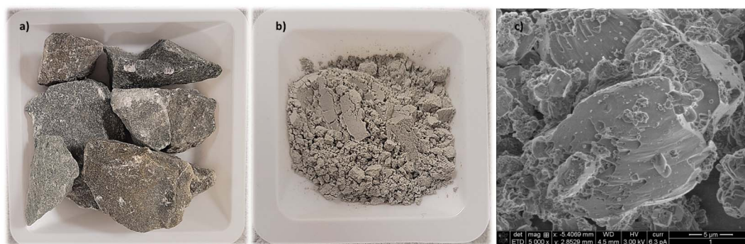
Fig. 8 (a) Uncrushed olivine; (b) olivine crushed to a powder; (c) SEM analysis of the crushed olivine.
