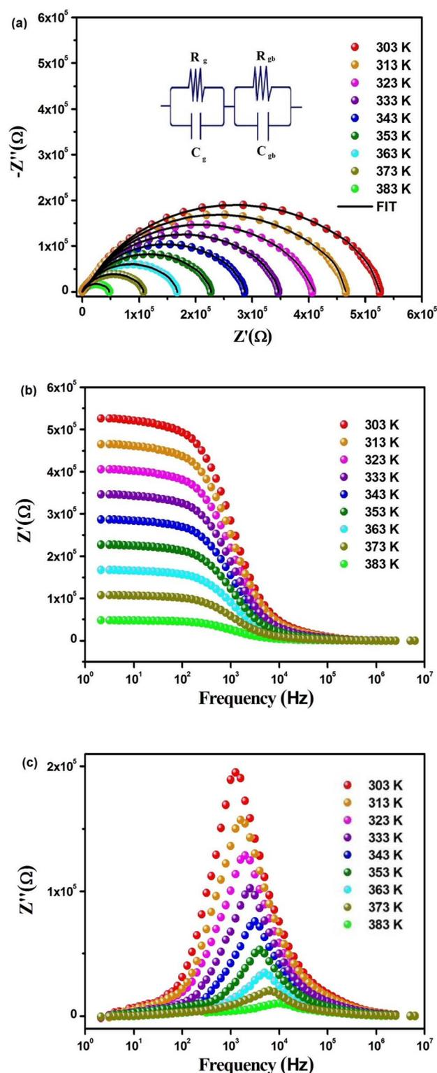
Fig. 6 (a) Adjusted Cole–Cole diagrams for  $\text{Cs}_2\text{TiBr}_6$  at various temperatures, with corresponding equivalent circuits illustrated in the inset. Temperature-dependent variation of (b)  $Z'(f)$  and (c)  $Z''(f)$ .
