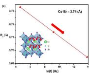
Fig. 9 (a) Variation of  $\sigma_{ac}(f)$  at different temperatures. (b)  $\sigma_{ac}$  vs. 1000/Tplot of  $Cs_2TiBr_6$ . (c) Variation of s and (1 - s) with temperature. (d) The temperature dependency of the  $ln(\sigma_{ac})$  at various frequencies. (e) Frequency-dependent of  $R_{\omega}$
