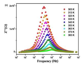
Fig. 6 (a) Adjusted Cole–Cole diagrams for  $Cs_2TiBr_6$  at various temperatures, with corresponding equivalent circuits illustrated in the inset. Temperature-dependent variation of (b) Z'(f) and (c) Z''(f).
