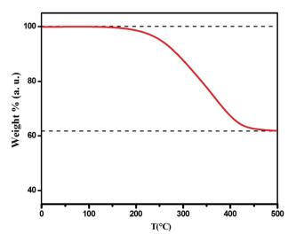
Fig. 3 TG data of Cs<sub>2</sub>TiBr<sub>6</sub> in the temperature range of 0-500 °C.
