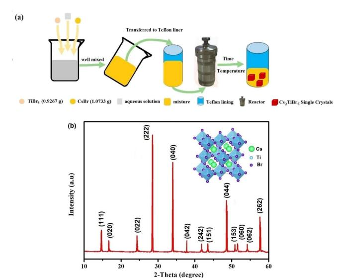
Fig. 1 (a) Schematic illustration of the slow cooling method to obtain  $Cs_2TiBr_6$  SCs. (b) Powder X-ray diffraction pattern of  $Cs_2TiBr_6$  obtained at ambient temperature within the  $2\theta$  range of  $10-60^\circ$ . The inset displays the arrangement of  $Cs_2TiBr_6$  in the crystal lattice.
