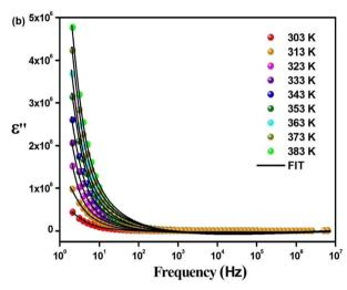
Fig. 7 Temperature-dependent of (a)  $\varepsilon'(f)$  and (b)  $\varepsilon''(f)$  for  $Cs_2TiBr_6$ .
