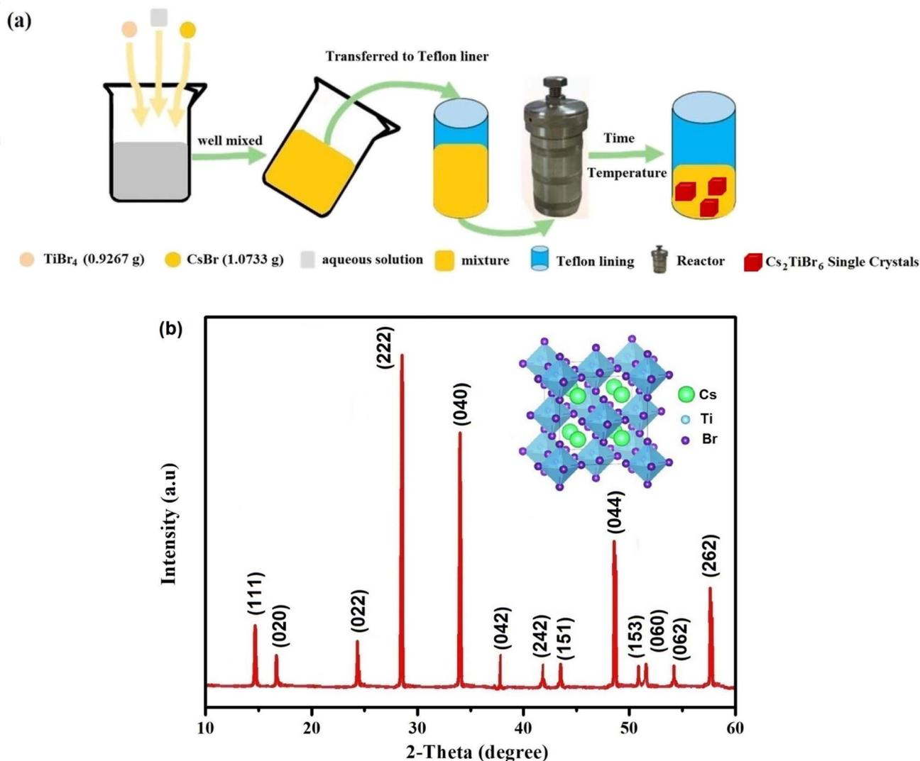
Fig. 1 (a) Schematic illustration of the slow cooling method to obtain  $\text{Cs}_2\text{TiBr}_6$  SCs. (b) Powder X-ray diffraction pattern of  $\text{Cs}_2\text{TiBr}_6$  obtained at ambient temperature within the  $2\theta$  range of  $10\text{--}60^\circ$ . The inset displays the arrangement of  $\text{Cs}_2\text{TiBr}_6$  in the crystal lattice.
