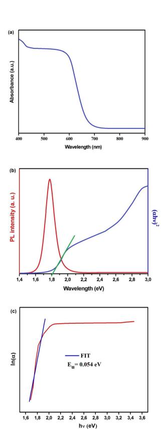
Fig. 4 (a) Absorption, (b) photoluminescence spectra and Tauc plot of  $Cs_2TiBr_6$ . (c)  $ln(\alpha)$  vs.  $h\nu$  (eV) of  $Cs_2TiBr_6$ .
