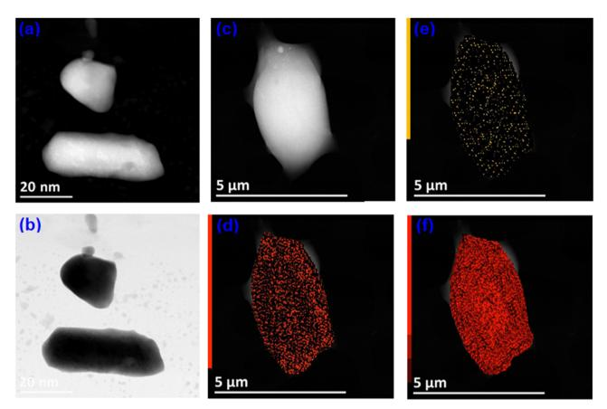
Fig. 2 (a), (b) STEM-HAADF image of  $Cs_2TiBr_6$ . (c)—(f) EDS mapping of Cs, Ti and Br in different colors.
