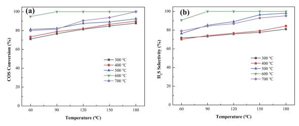
Fig. 3 (a) COS conversion, (b)  $H_2S$  selectivity of 3%  $Sm_2O_3$ -Ce- $O_x$ @Zr $O_2$  catalysts under different calcination temperatures.
