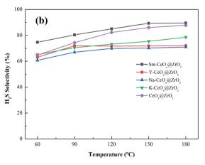
Fig. 1 (a) COS conversion, (b) H<sub>2</sub>S selectivity of M-Ce-O<sub>x</sub>@ZrO<sub>2</sub> catalysts.
