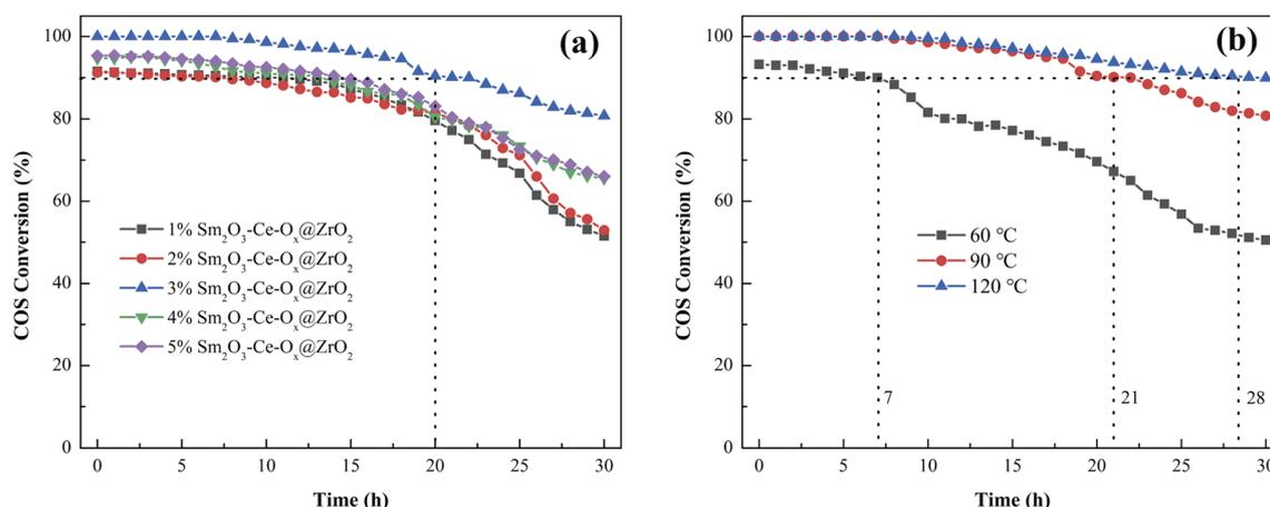
Fig. 5 Stability of Sm<sub>2</sub>O<sub>3</sub>-Ce-O<sub>x</sub>@ZrO<sub>2</sub> catalyst: (a) different Sm contents, (b) different reaction temperature.
