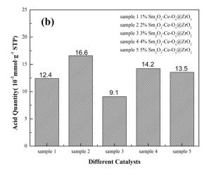
Fig. 10 (a) NH<sub>3</sub>-TPD profiles and (b) acid quantity of Sm-Ce-O<sub>x</sub>@ZrO<sub>2</sub> catalysts with different Sm contents
