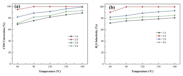
Fig. 4 (a) COS conversion, (b) H<sub>2</sub>S selectivity and of 3% Sm<sub>2</sub>O<sub>3</sub>-Ce-O<sub>v</sub>@ZrO<sub>2</sub> catalysts under different calcination time.
