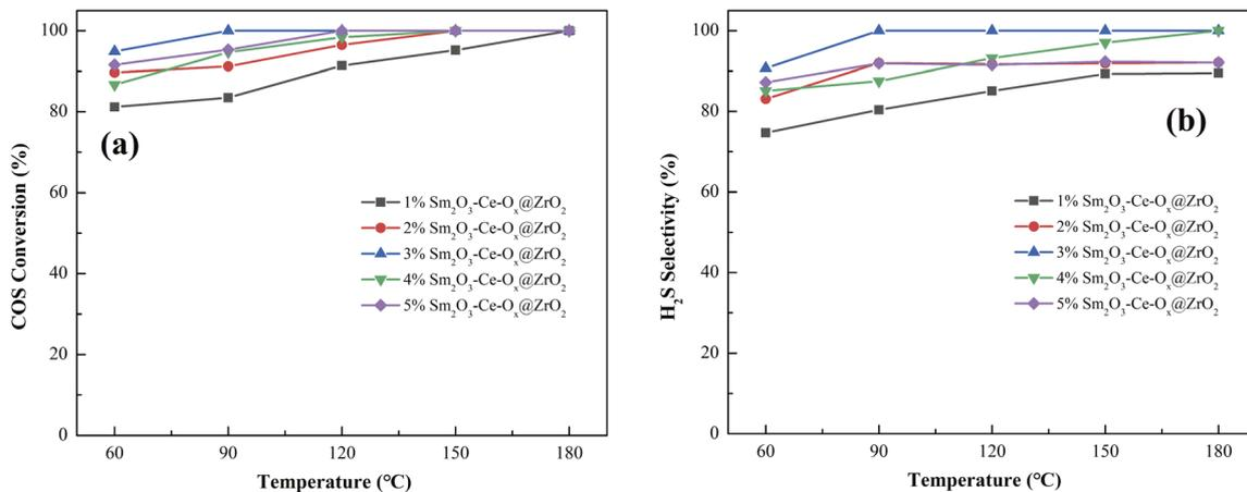
Fig. 2 (a) COS conversion, (b) H<sub>2</sub>S selectivity of Sm-Ce-O<sub>x</sub>@ZrO<sub>2</sub> catalysts with different Sm contents.
