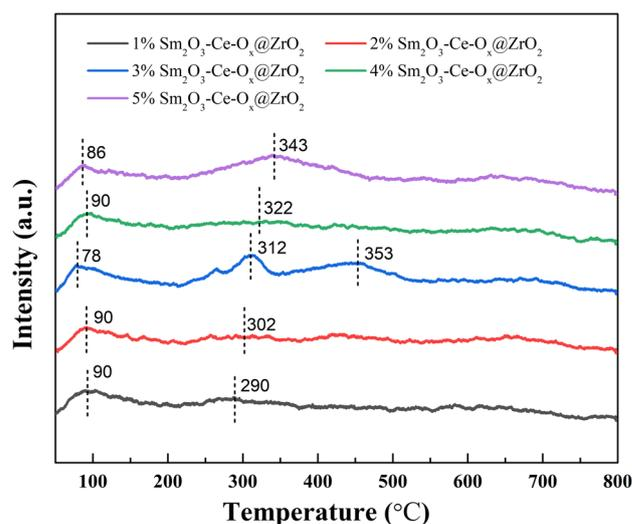
Fig. 11 CO<sub>2</sub>-TPD profiles of Sm<sub>2</sub>O<sub>3</sub>-Ce-O<sub>x</sub>@ZrO<sub>2</sub> catalysts with different Sm contents.
