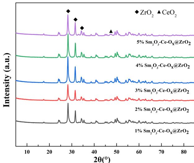
Fig. 6 XRD patterns of Sm<sub>2</sub>O<sub>3</sub>-Ce-O<sub>x</sub>@ZrO<sub>2</sub> catalysts with different Sm contents.
