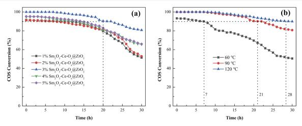
Fig. 5 Stability of Sm<sub>2</sub>O<sub>3</sub>-Ce-O<sub>x</sub>@ZrO<sub>2</sub> catalyst: (a) different Sm contents, (b) different reaction temperature
