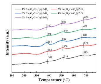
Fig. 12  $H_2$ -TPR profiles of  $Sm_2O_3$ -Ce- $O_x$ @Zr $O_2$  catalysts with different Sm contents.
