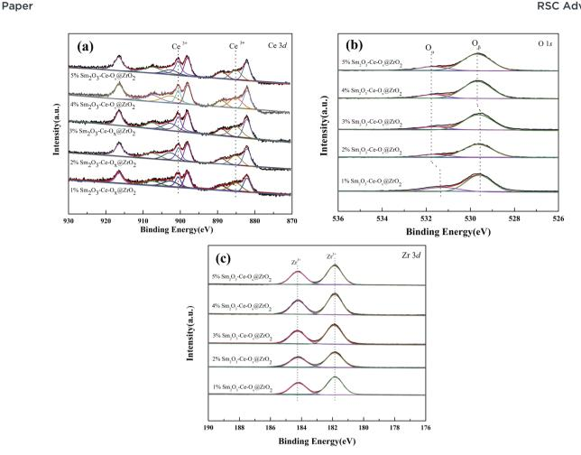
XPS profiles of Sm<sub>2</sub>O<sub>3</sub>-Ce-O<sub>x</sub>@ZrO<sub>2</sub> catalysts with different Sm contents (a) Ce 3d, (b) O 1s, (c) Zr 3d.
