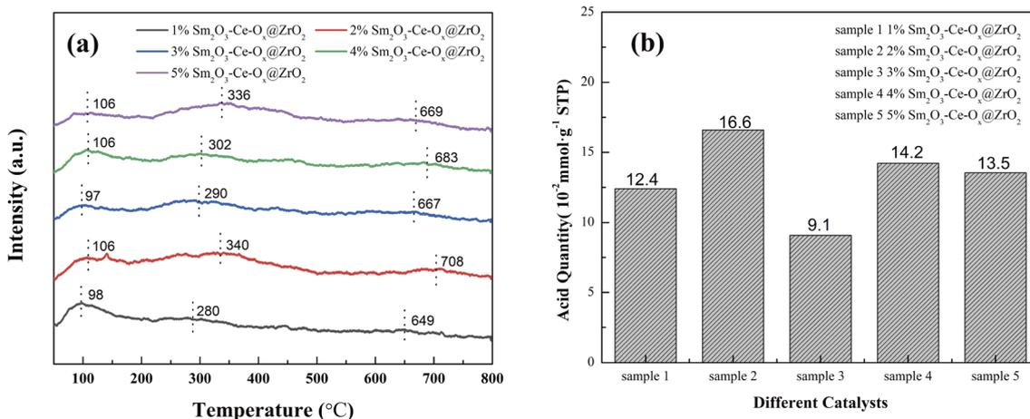
Fig. 10 (a) NH<sub>3</sub>-TPD profiles and (b) acid quantity of Sm-Ce-O<sub>x</sub>@ZrO<sub>2</sub> catalysts with different Sm contents.
