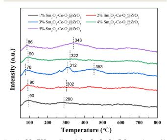
Fig. 11  $CO_2$ -TPD profiles of  $Sm_2O_3$ -Ce- $O_x@ZrO_2$  catalysts with different Sm contents.
