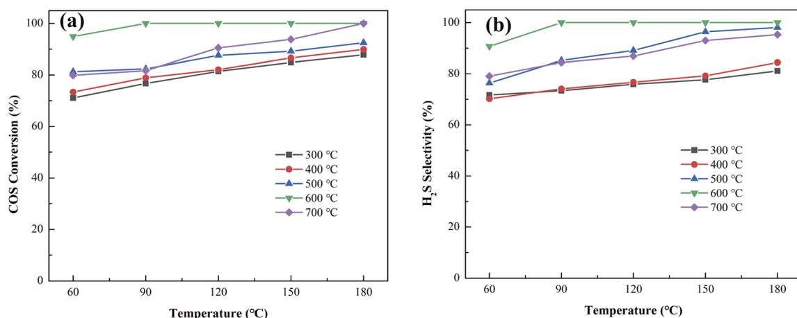
Fig. 3 (a) COS conversion, (b) H<sub>2</sub>S selectivity of 3% Sm<sub>2</sub>O<sub>3</sub>-Ce-O<sub>x</sub>@ZrO<sub>2</sub> catalysts under different calcination temperatures.
