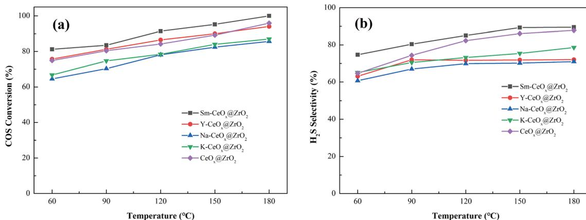
Fig. 1 (a) COS conversion, (b) H<sub>2</sub>S selectivity of M-Ce-O<sub>x</sub>@ZrO<sub>2</sub> catalysts.
