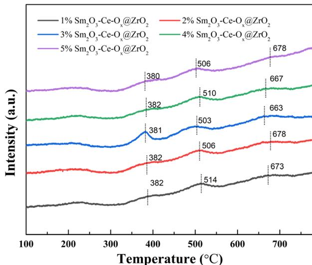
Fig. 12 H<sub>2</sub>-TPR profiles of Sm<sub>2</sub>O<sub>3</sub>-Ce-O<sub>x</sub>@ZrO<sub>2</sub> catalysts with different Sm contents.
