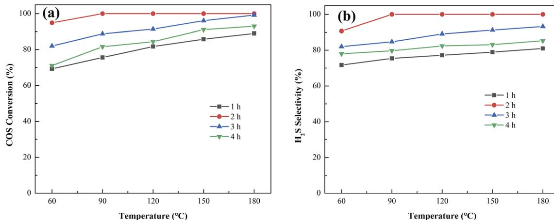
Fig. 4 (a) COS conversion, (b) H<sub>2</sub>S selectivity and of 3% Sm<sub>2</sub>O<sub>3</sub>-Ce-O<sub>x</sub>@ZrO<sub>2</sub> catalysts under different calcination time.
