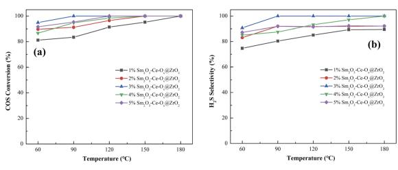
Fig. 2 (a) COS conversion, (b) H<sub>2</sub>S selectivity of Sm-Ce-O<sub>x</sub>@ZrO<sub>2</sub> catalysts with different Sm contents.
