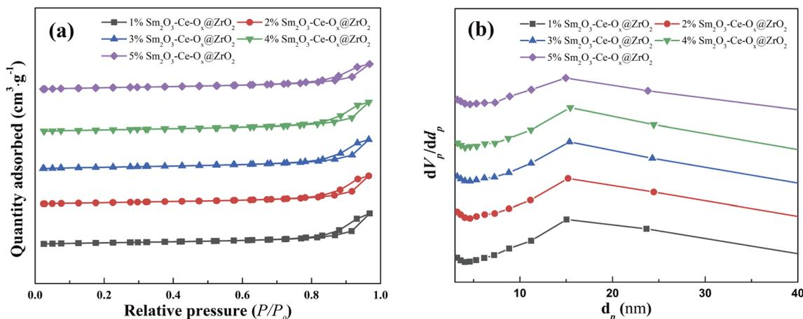
Fig. 7 (a) N<sub>2</sub> adsorption–desorption and (b) pore size distribution curves of Sm<sub>2</sub>O<sub>3</sub>-Ce-O<sub>x</sub>@ZrO<sub>2</sub> catalysts with different Sm contents.
