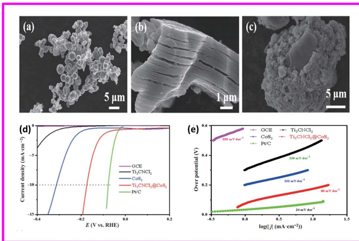
Fig. 7 SEM images of (a)  $\text{CoS}_2$  microspheres (b)  $\text{Ti}_3\text{CNCl}_2$  nanosheets (c)  $\text{Ti}_3\text{CNCl}_2@CoS_2$  core shell nanostructures (d) polarization curves (e) corresponding Tafel slopes. Reproduced with permission.<sup>72</sup>
