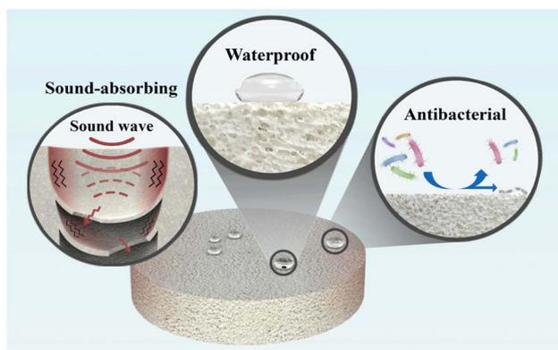
Fig. 9 Mechanism of the multifunctional ceramic foams.
