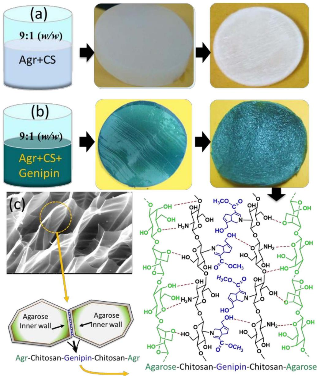
Fig. 6 Aerogel membrane preparation schematics: (a) uncrosslinked chitosan, (b) genipin-crosslinked chitosan, and (c) genipin-crosslinked chitosan with agarose H-bonding to the inner walls of CS. Reproduced with permission from<sup>138</sup> Copyright (2015), ACS.
