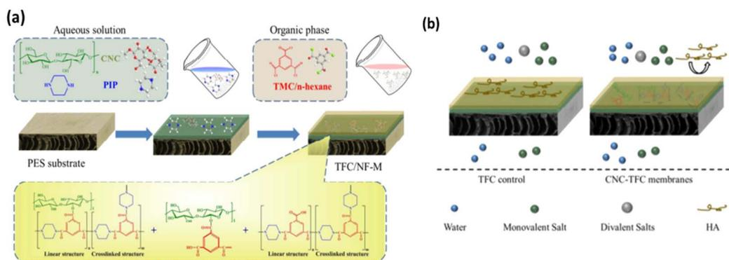
Fig. 2 (a) Synthetic scheme of the CNC-TFC membrane. (b) Adsorption mechanism of CNC-TFC membranes for metal ions. Reproduced with permission.<sup>68</sup> Copyright (2018), ACS.
