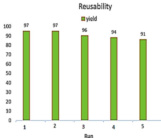
Fig. 10 The reusability of the  $\text{Fe}_3\text{O}_4@CS-SB-CaMgFe_2O_4$  nanocatalyst.
