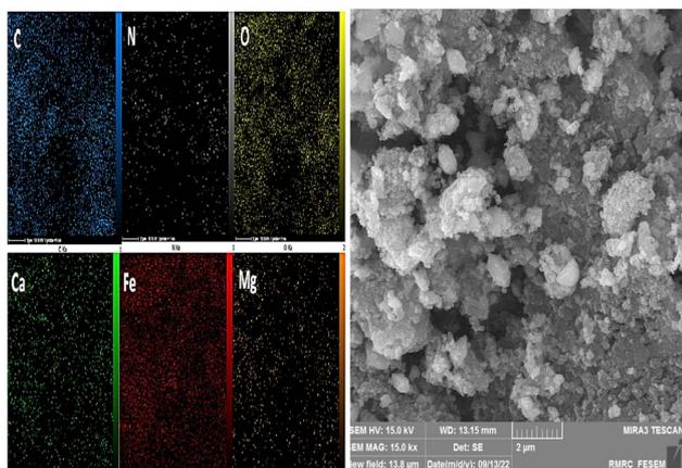
Fig. 7 Mapping images of the  $\text{Fe}_3\text{O}_4@CS-SB-CaMgFe_2\text{O}_4$  nanocatalyst.
