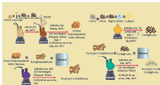
Fig. 1 The stepwise preparation of Fe<sub>3</sub>O<sub>4</sub>@CS-SB-CaMgFe<sub>2</sub>O<sub>4</sub> magnetic nanoparticles.
