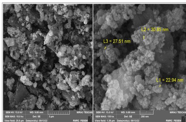
Fig. 5 FE-SEM images of the  $\text{Fe}_3\text{O}_4@CS-SB-CaMgFe_2\text{O}_4$  nanocatalyst.
