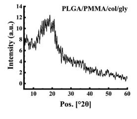
Fig. 5 XRD patterns of components of electrospun PLGA/PMMA/col/gly nanofibers loaded with SCLE.
