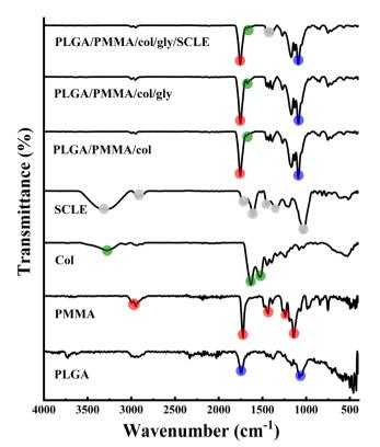
Fig. 4 FTIR spectra of individual components of the electrospun PLGA/PMMA/col/gly/SCLE nanofibers. The main characteristic peaks of each spectrum are highlighted to demonstrate changes in the formed nanofibers.
