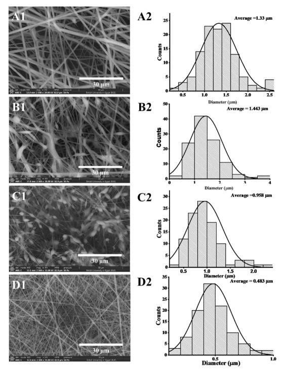
Fig. 3 Scanning electron microscopy images, captured at a magnification of 2500×, showing the morphology of electrospun PLGA/PMMA/col/ gly/SCLE nanofibers: (A1) PLGA (15%)/PMMA (10%) (F1), (B1) PLGA/PMMA/col (1%) (F6), (C1) PLGA/PMMA/col/gly (0.1%) (F7), and (D1) PLGA/PMMA/ col/gly (0.1%)/SCLE (1%) (F11). A2, B2, C2, and D2 represent diameter distribution histograms of F1, F6, F7, and F11, respectively.
