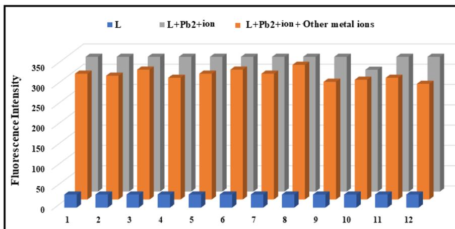
Fig. 13 Fluorescence interference study of **L** (where 1 = **L**, 2 =  $\text{Fe}^{3+}$ , 3 =  $\text{Cr}^{3+}$ , 4 =  $\text{Ni}^{2+}$ , 5 =  $\text{Cd}^{2+}$ , 6 =  $\text{Ni}^{2+}$ , 7 =  $\text{Zn}^{2+}$ , 8 =  $\text{Pb}^{2+}$ , 9 =  $\text{Ag}^+$ , 10 =  $\text{Al}^{3+}$ , 11 =  $\text{Mn}^{2+}$  and 12 =  $\text{Hg}^{2+}$ ). Excitation wavelength was 340 nm and emission maxima were at 417 nm.
