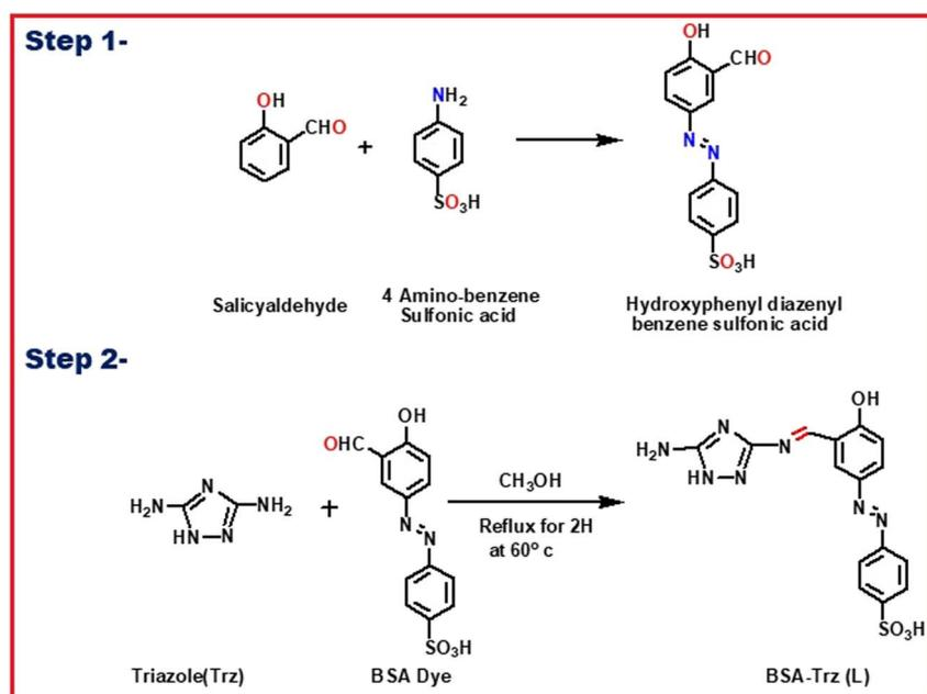
Scheme 1 Synthetic procedure of the probe **L**.
