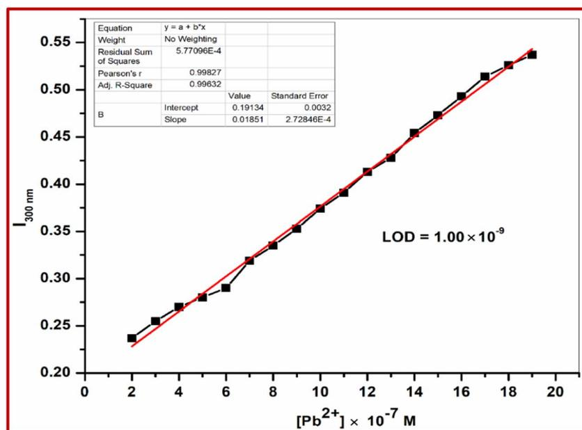
Fig. 6 Detection limit for Pb<sup>2+</sup> from absorption spectra in CH<sub>3</sub>OH–H<sub>2</sub>O (1 : 2).
