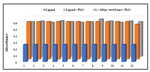
Fig. 7 Absorbance competitive experiment of L with other metal ions (where 1 = L,  $2 = Fe^{3+}$ ,  $3 = Cr^{3+}$ ,  $4 = Ni^{2+}$ ,  $5 = Cd^{2+}$ ,  $6 = Ni^{2+}$ ,  $7 = Zn^{2+}$ ,  $8 = Cr^{3+}$ ,  $1 = Ni^{2+}$ ,  $1 = Ni^{2+$  $Pb^{2+}$ ,  $9 = Ag^{+}$ ,  $10 = Al^{3+}$ ,  $11 = Mn^{2+}$  and  $12 = Hg^{2+}$ ). Wavelength was monitored at 300 nm.
