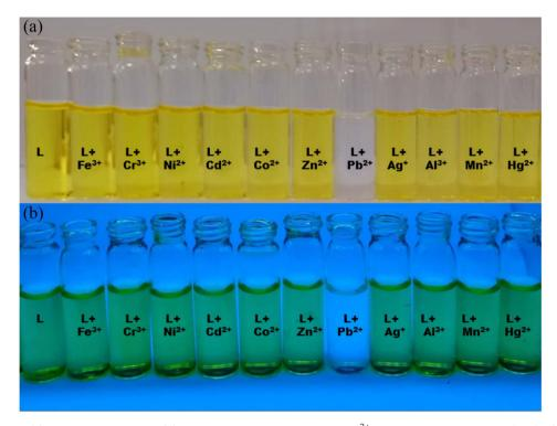
Fig. 2 Colour changes (a) to the naked eye and (b) under UV light of ligand L with  $Pb^{2+}$  ions and other cations in  $CH_3OH/H_2O$  (1:2).
