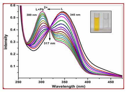
Fig. 5 UV-visible titration of L with Pb<sup>2+</sup> in CH<sub>3</sub>OH-H<sub>2</sub>O (1:2). Inset: colour change of L on addition of 2 equiv. of Pb<sup>2+</sup>.
