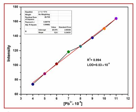
Fig. 12 Detection limit for  $Pb^{2+}$  from emission spectra in  $CH_3OH-H_2O$  (1:2).
