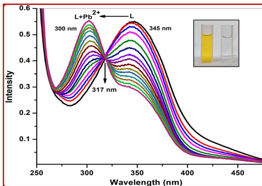
Fig. 5 UV-visible titration of L with Pb<sup>2+</sup> in CH<sub>3</sub>OH–H<sub>2</sub>O (1 : 2). Inset: colour change of L on addition of 2 equiv. of Pb<sup>2+</sup>.
