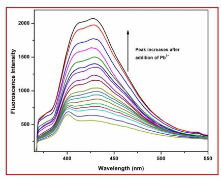
Fig. 14 Fluorescence spectra of L in the presence of 3 equiv. of Pb<sup>2+</sup> in aqueous bovine serum albumin medium.
