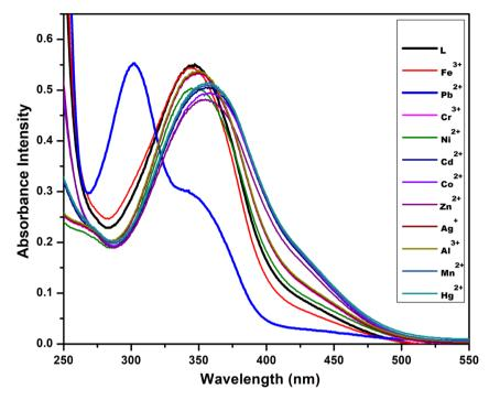
Fig. 3 Absorption spectra of L (10  $\mu$ M) in the presence of 3 equiv. of different metal ions in CH<sub>3</sub>OH-H<sub>2</sub>O (1:2).
