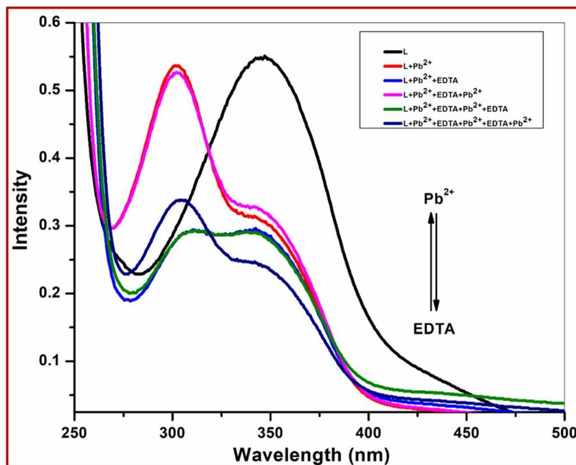
Fig. 9 Reversibility study of L complex with Na<sub>2</sub> EDTA.
