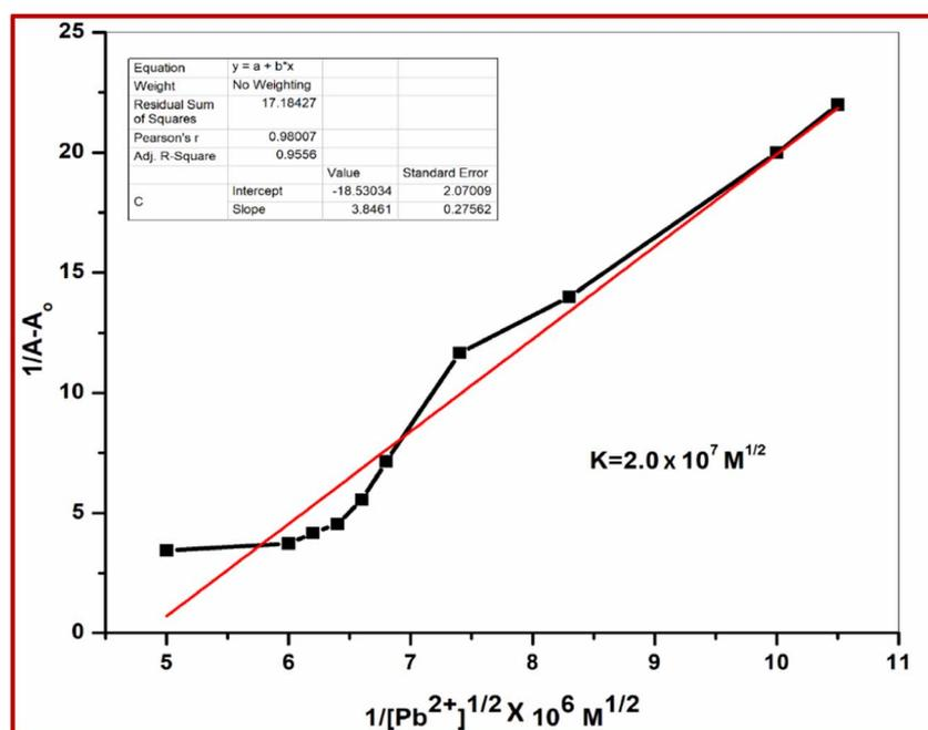
Fig. 8 Binding constants of L-Pb<sup>2+</sup> complex.
