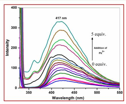
Fig. 11 Fluorescence titration of L with different concentrations of metal ions in CH<sub>3</sub>OH-H<sub>2</sub>O (1:2) on excitation at 310 nm.
