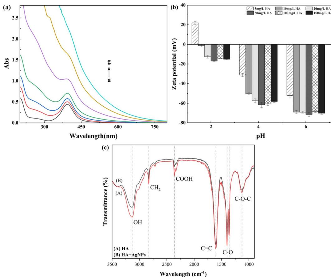
Fig. 4 (a) Surface plasmon resonance absorption of different concentrations of HA with AgNPs.  $[\text{AgNPs}] = 3.774 \text{ mg L}^{-1}$ , a–g:  $[\text{HA}] = 0, 5, 10, 20, 50, 100, \text{ and } 150 \text{ mg L}^{-1}$ . (b) Effect of different concentrations of HA on the zeta potential of AgNPs. (c) Infrared spectra of AgNPs before and after the interaction with HA.
