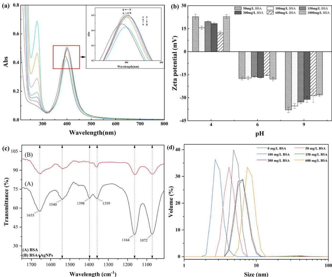
Fig. 2 (a) Surface plasmon resonance absorption of different concentrations of BSA with AgNPs. [AgNPs] =  $3.774 \text{ mg L}^{-1}$ , a–g: [BSA] = 0, 50, 100, 150, 300, 600, and 1000  $\text{mg L}^{-1}$ . (b) Effect of different concentrations of BSA on the zeta potential of AgNPs. (c) Infrared spectra of AgNPs before and after the interaction with BSA. (d) Effect of different concentrations of BSA on the average particle size of AgNPs.
