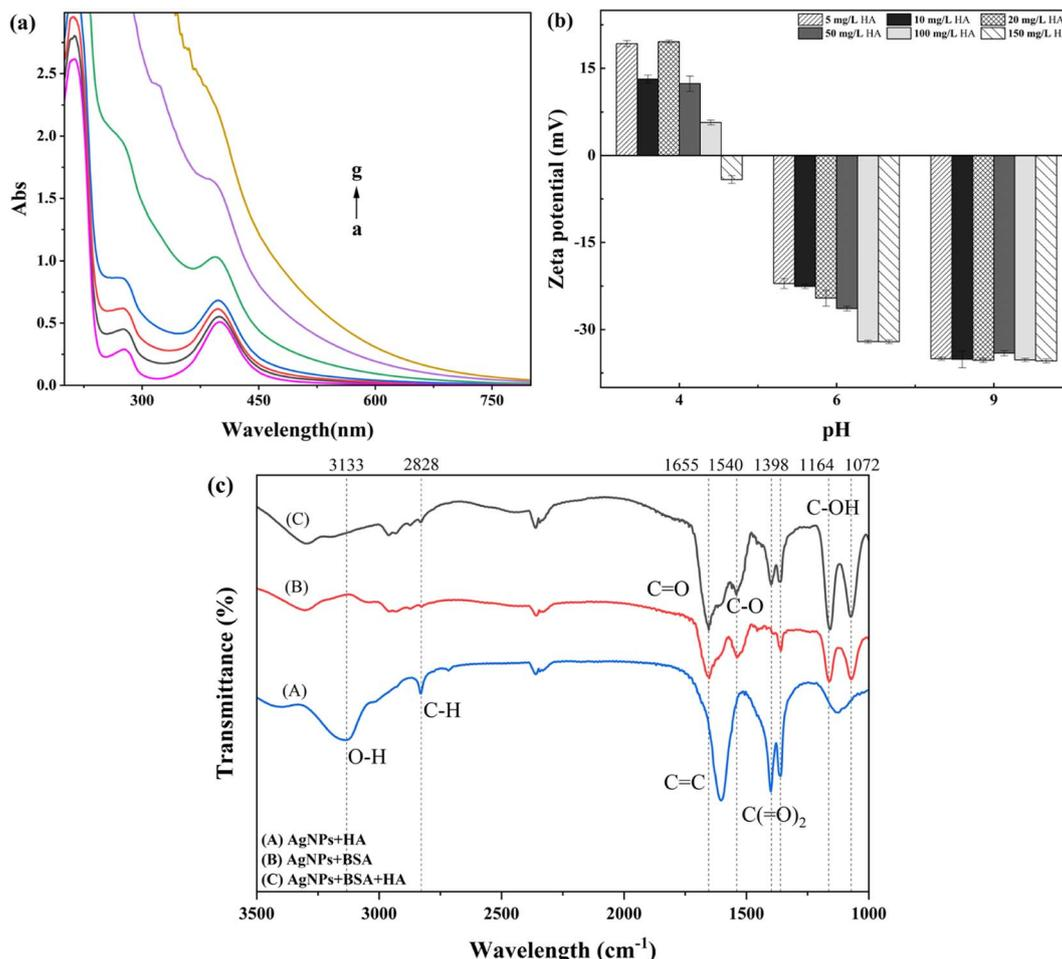
Fig. 5 (a) UV-vis spectra of AgNP-BSA complexes with different concentrations of HA. [AgNPs] = 3.774 mg L<sup>-1</sup>, [BSA] = 300 mg L<sup>-1</sup>, a-g: [HA] = 5, 10, 20, 50, 100, and 150 mg L<sup>-1</sup>. (b) Effects of different concentrations of HA on the zeta potential of AgNP-BSA complexes. (c) Infrared spectra of AgNP-BSA before and after HA addition.
