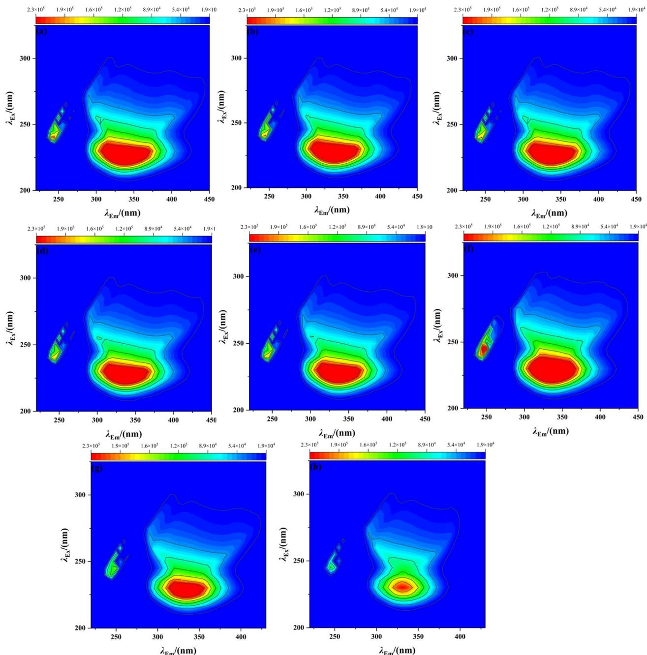
Fig. 3 Three-dimensional fluorescence spectra of AgNPs with BSA at different concentrations. [BSA] =  $300 \text{ mg L}^{-1}$ , a–h: [AgNPs] = 0, 0.3774, 0.4718, 0.9435, 1.258, 1.887, 4.718, and  $9.435 \text{ mg L}^{-1}$ .
