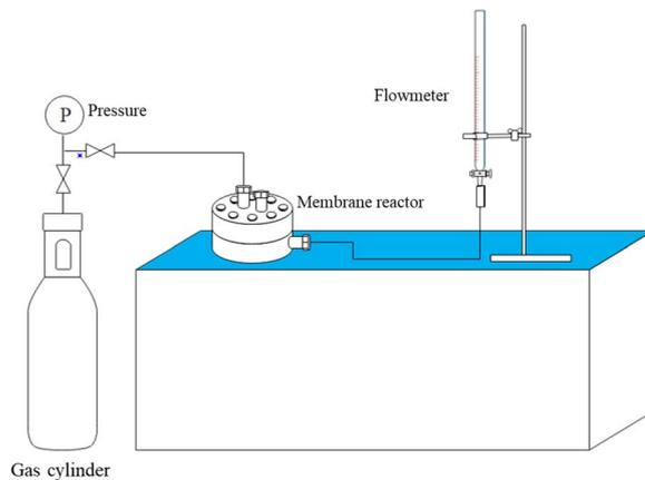
Fig. 2 Schematic of a single gas permeation test.
