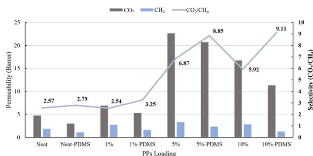
Fig. 8 Separation performance for CO<sub>2</sub>/CH<sub>4</sub>.
