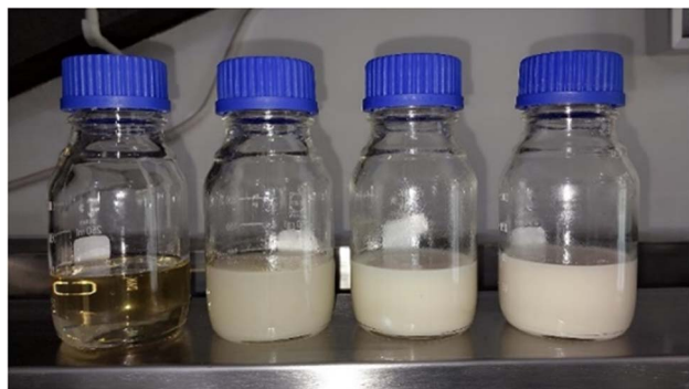
Fig. 3 Dope solution PSf and PSf/PPs 1, 5, and 10 wt%.
