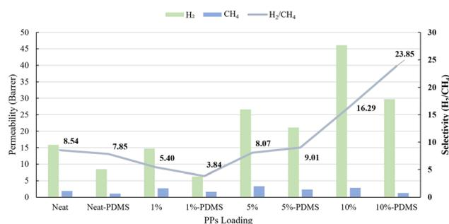
Fig. 9 Separation performance for H<sub>2</sub>/CH<sub>4</sub>.
