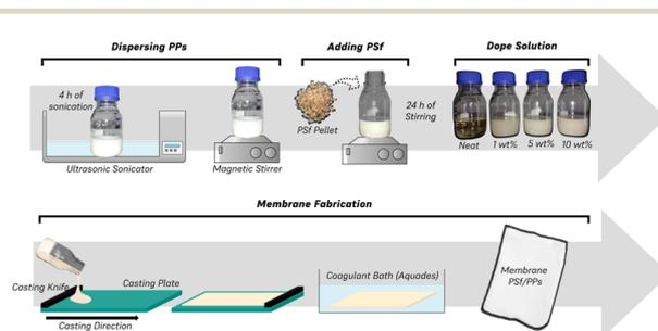
Fig. 1 The preparation scheme for PSf/PPs membrane.
