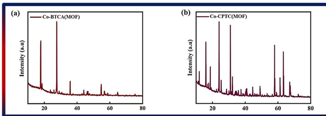
Fig. 2 Structural interpretation: (a) XRD of Co-BTCA(MOF), (b) XRD Co-CPTC(MOF).
