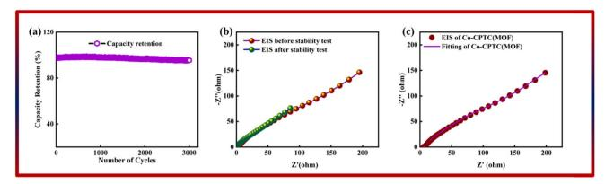
Fig. 8 (a) Stability of Co-CPTC(MOF)//AC. (b) EIS before and after stability test. (c and d) Fitted model of EIS of Co-CPTC(MOF).
