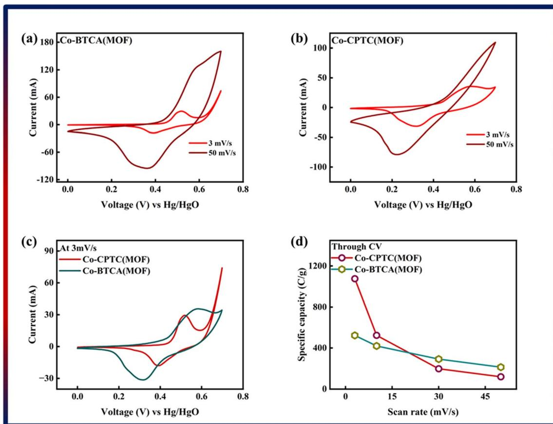
Fig. 3 (a) Cyclic voltammetry of Co-BTCA(MOF). (b) Cyclic voltammetry of Co-CPTC(MOF). (c) Comparison of both MOF CV curves at 3 mV s<sup>-1</sup>. (d) Specific capacity through CV of both MOFs.
