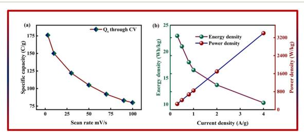
Fig. 7 (a) Specific capacity of Co-CPTC(MOF)//AC through GCD. (b) Energy density and power density of Co-CPTC(MOF)//AC.
