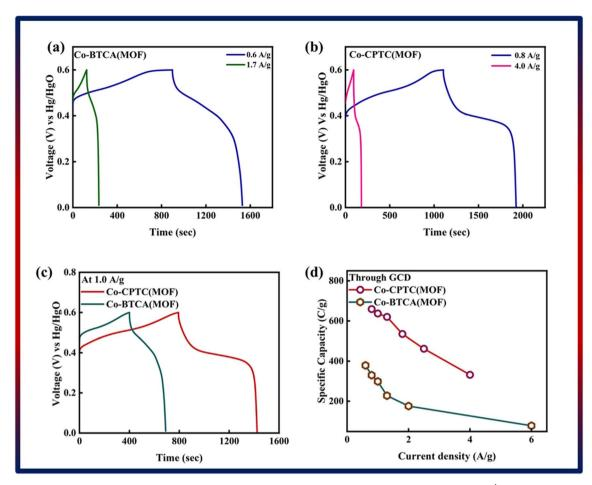
Fig. 4 GCD of (a) Co-BTCA(MOF) and (b) Co-CPTC(MOF). (c) Comparison of both MOF GCD curves at  $1.0~{\rm A~g^{-1}}$ . (d) Specific capacity through GCD of both MOFs.
