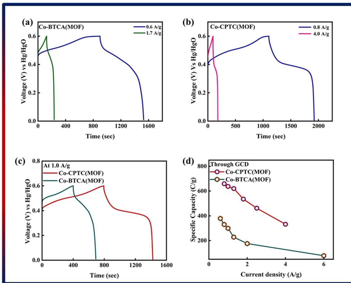
Fig. 4 GCD of (a) Co-BTCA(MOF) and (b) Co-CPTC(MOF). (c) Comparison of both MOF GCD curves at 1.0 A g<sup>-1</sup>. (d) Specific capacity through GCD of both MOFs.
