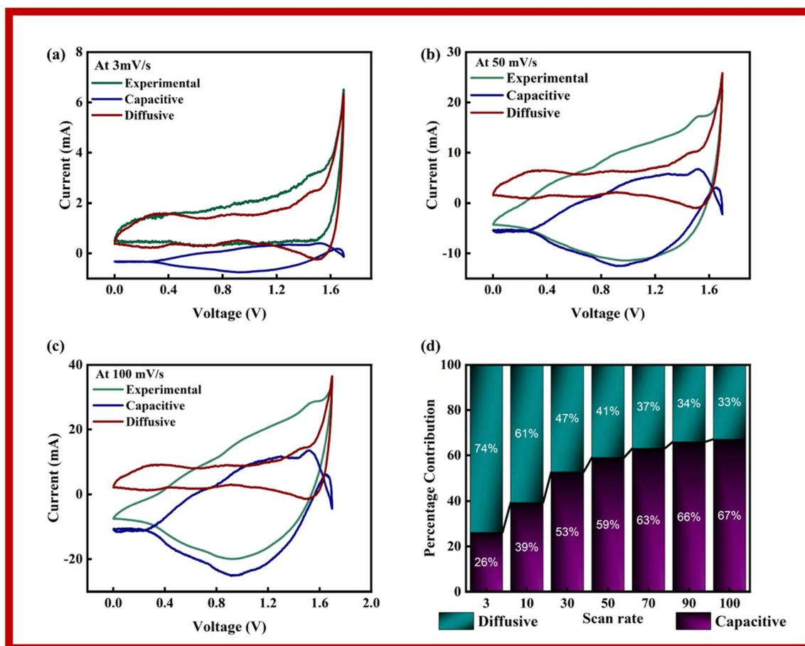
Fig. 9 Contribution of capacitive and diffuse elements to the total CV spectrum of Co-CPTC(MOF) at (a)  $3 \text{ mV s}^{-1}$ , (b)  $50 \text{ mV s}^{-1}$ , (c)  $100 \text{ mV s}^{-1}$ . (d) Percentage of capacitive and diffusive contribution at various scan rates.
