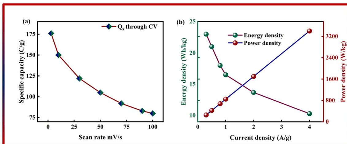
Fig. 7 (a) Specific capacity of Co-CPTC(MOF)//AC through GCD. (b) Energy density and power density of Co-CPTC(MOF)//AC.
