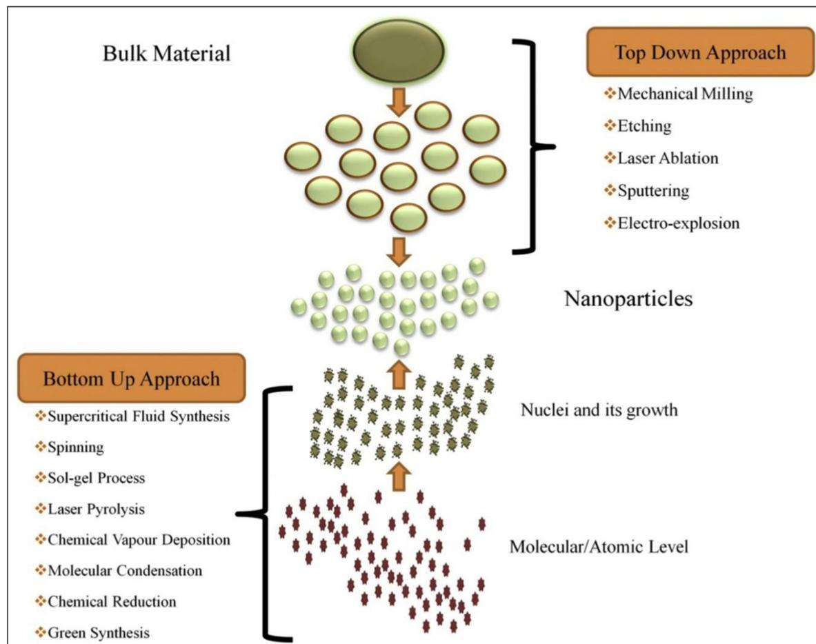
Fig. 5 Schematic drawing related to the synthesis of nanomaterials (NPs) via top-down and bottom-up approaches (Reprinted from<sup>84</sup> with permission from Elsevier).
