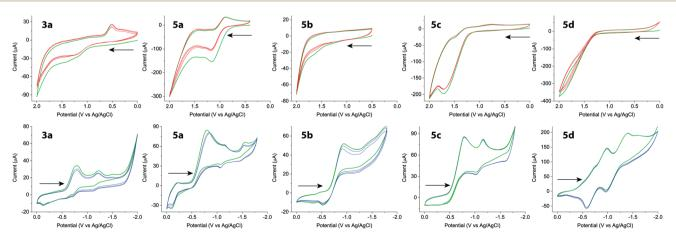
Fig. 3 Cyclic voltammograms of compounds 3a, 5a-d scanned in positive (top) and negative (bottom) potential windows, respectively. Experimental conditions:  $CH_2Cl_2$  as solvent,  $Bu_4NBF_4$  (0.1 M) as electrolyte, glassy carbon as the working electrode, Ag/AgCl as the reference electrode, and Pt wire as the counter electrode. Scan rate  $= 0.20 \text{ V s}^{-1}$ .
