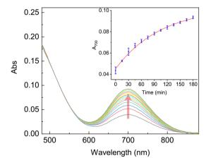
Fig. 6 UV-vis spectra of **5a** (55.0  $\mu$ M in CHCl<sub>3</sub>) mixed with TFA (4.0 mole equivalents) recorded at different time intervals. The arrow indicates the trend of change. Inset: plot of the absorbance at 700 nm ( $A_{700}$ ) as a function of time (t, min). The red-color trace shows the curve fitting with a mono-exponential nonlinear equation,  $y=y_0+C\times e^{-kx}$ , where  $k=105.32\pm7.04$  min<sup>-1</sup> and  $R^2=0.998$ .
