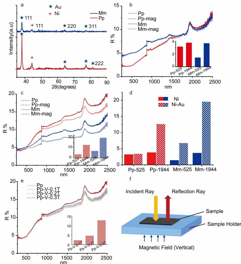
Fig. 3 (a) XRD results of Ni–Au<sub>30</sub> BWs; (b) reflectance spectra of Ni BWs; (c) reflectance spectra of Ni–Au<sub>30</sub> BWs; (d) comparison of magneto-optical effect differences for various samples; (e) Pp–Ni–Au<sub>30</sub> BWs' reflectance spectra under different magnetic fields; (f) schematic of the experimental set-up for reflectance measurements under various applied magnetic fields.
