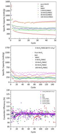
Fig. 8 Cycling performance of BGC, NBGC, MnO<sub>2</sub>/NBGC at various MnO<sub>2</sub> loadings and pure synthesized MnO<sub>2</sub>: (a) cycling at a current density of 186 mA g $^{-1}$ , (b) cycling at a current density of 774 mA g $^{-1}$  and (c) their corresponding coulombic efficiency at a current density of 774 mA g $^{-1}$ .
