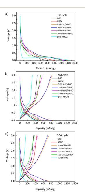
Fig. 7 The voltage profiles of bagasse-derived carbon material (BGC), N-doping bagasse-derived carbon (NBGC), and  $MnO_2/NBGC$  composites with various  $MnO_2$  loadings at the (a) 1st cycle, (b) 2nd cycle, and (c) 50th cycle.
