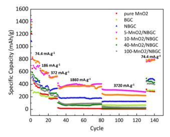
Fig. 9 Rate performance of bagasse-derived carbon material (BGC), N-doping bagasse-derived carbon (NBGC), MnO<sub>2</sub>/NBGC carbon composite with various MnO2 loading concentrations and the pure hydrothermally synthesized MnO<sub>2</sub>
