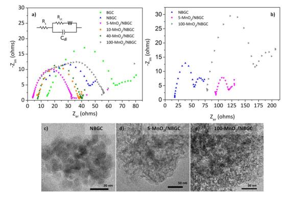
Fig. 10 Electrochemical impedance of (a) the fresh carbon composite anode electrodes and (b) carbon composite anode electrodes after cycling at 774 mA  $\rm g^{-1}$  for 150 cycles; the TEM images of some spent carbon composite electrodes: (c) NBGC, (d) 5-MnO<sub>2</sub>/NBGC, and (e) 100-MnO<sub>2</sub>/NBGC.
