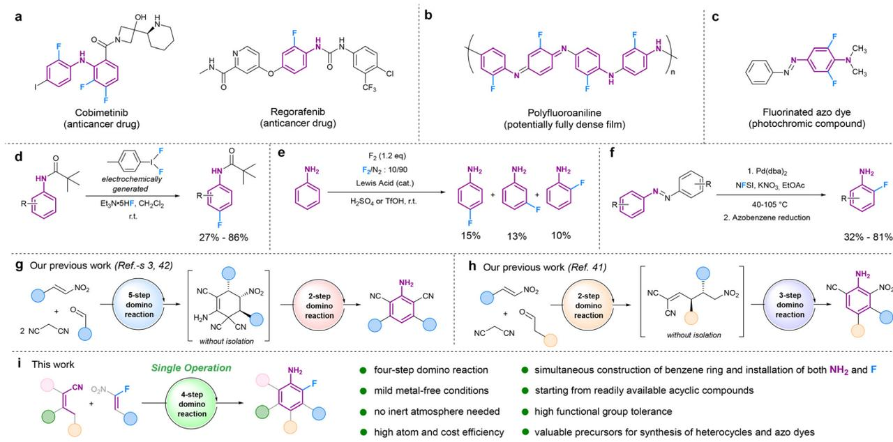
**Fig. 1** (a) Examples of fluoroaniline-containing drug compounds; (b) structure of polyfluoroaniline; (c) fluorinated azo dye; (d–f) literature known fluorinations of anilines; (g and h) previously reported domino approaches toward functionalized anilines by our research group; (i) *this work*: new straightforward four-step domino reaction toward functionalized fluoroaniline compounds.
