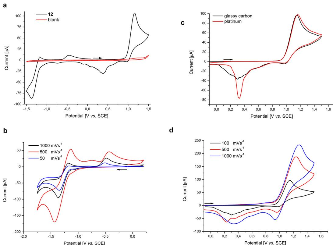
**Fig. 4** Cyclic voltammetry of **12** (5 mM). (a) at  $100 \text{ mV s}^{-1}$  in DCM with  $n\text{-Bu}_4\text{NPF}_6$  (0.1 M); (b) at different scan rates in DCM with  $n\text{-Bu}_4\text{NPF}_6$  (0.1 M) in oxidative potential regimes; (c) at  $100 \text{ mV s}^{-1}$  in DCM with  $n\text{-Bu}_4\text{NPF}_6$  (0.1 M) at a glassy carbon (black) or a platinum (red) working electrode; (d) at different scan rates in DCM with  $n\text{-Bu}_4\text{NPF}_6$  (0.1 M) in reductive potential regimes.
