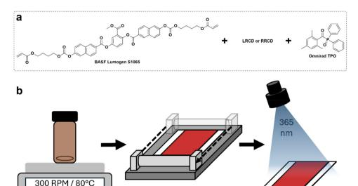
Fig. 2 (a) The CLC mixture components. (b) The schematic of the coating procedure of the CLC mixture on a PET substrate, followed by free radical photopolymerization of diacrylates.
