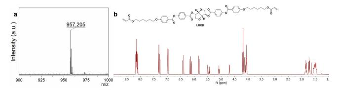
Fig. 1 (a) MALDI-TOF-MS measurement of LRCD. (b) The <sup>1</sup>H-NMR spectrum of LRCD in CDCl<sub>3</sub>
