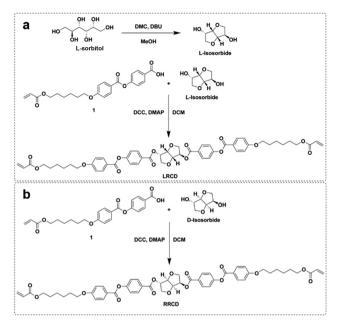
Scheme 2 a) Synthesis of L-isosorbide and LRCD. (b) Synthesis of
