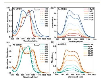
Fig. 5 Normalized absorption spectra of (a) Az-BSQ-S and (c) Az-BSQ-D (10 μM) in THF/hexane mixed solvents with hexane volume fractions ranging from 10% to 90%. Absorption spectra of (b) Az-BSQ-S ( $f_{\text{hexane}} = 60\%$ ) and (d) Az-BSQ-D ( $f_{\text{hexane}} = 50\%$ ) at different concentrations in the THF/hexane system.
