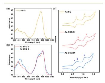
Fig. 3 UV-vis/NIR absorption spectra of (a) Az-SQ ( $10^{-5}$  M) and (b) Az-BSQ-S and Az-BSQ-D (5  $\times$  10<sup>-6</sup> M) in THF. (c) Cyclic voltammetry curves of Az-SQ, Az-BSQ-S and Az-BSQ-D in DCM (TBAPF, was used as the supporting electrolyte and SCE as the reference electrode) in the positive voltage range.
