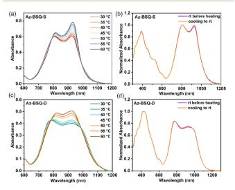
Fig. 6 Temperature-dependent absorption spectra of (a) Az-BSQ-S and (c) Az-BSQ-D during the heating process in the THF/hexane system (10  $\mu$ M,  $f_{hexane}$  = 60%). Absorption spectra of (b) Az-BSQ-S and (d) Az-BSQ-D before heating and after cooling to room temperature.
