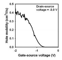
Fig. 6 Electrical characteristics of a DBAF TFT fabricated on a flexible PEN substrate in the inverted staggered (bottom-gate, top-contact) device architecture using an n-tetradecylphosphonic acid SAM as part of the gate dielectric, with the substrate held at a temperature of 80 °C during the semiconductor deposition. The effective charge-carrier mobility is  $0.4 \text{ cm}^2 \text{ V}^{-1} \text{ s}^{-1}$ .
