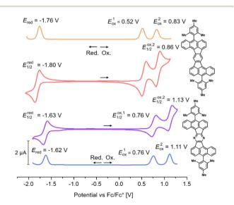
Fig. 3 Cyclic voltammograms (CV) and differential pulse voltammograms (DPV) of mes-DBAF (top) and mes-DBAF-N2 (bottom) in dichloromethane (c = 1 mM) using [Bu<sub>4</sub>N][PF<sub>6</sub>] (0.1 M) as electrolyte. CV scan speed 100 mV s<sup>-1</sup>; DPV: step size of 0.005 V, a modulation amplitude of 0.025 V a modulation time of 0.05 s and an interval time of 0.5 s.
