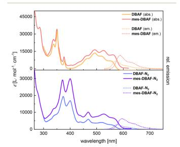
Fig. 2 UV/vis absorption (solid lines) and fluorescence (dashed lines) spectra of DBAF (red) and mes-DBAF (orange) (top) and DBAF-N $_2$  (blue) and mes-DBAF-N $_2$  (violet) (bottom), measured in o-DCB (DBAF and DBAF-N $_2$ ) or CH $_2$ Cl $_2$  (mes-DBAF) and mes-DBAF-N $_2$  at room temperature.
