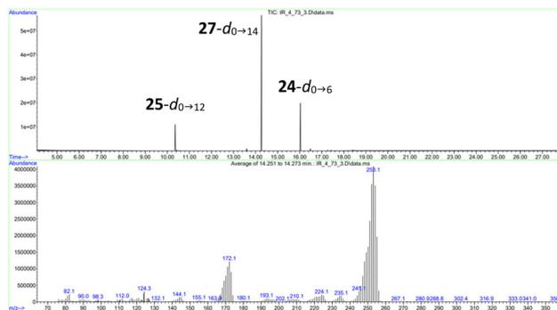
**Fig. 4** GCMS data from reaction of tetraphenylmethane **24** in C<sub>6</sub>D<sub>6</sub>. GC trace together with mass spectrum of **27** (*d*<sub>0</sub> → *d*<sub>14</sub>).
