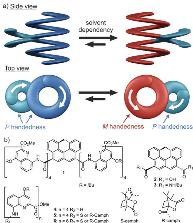
**Fig. 1** (a) Cartoon representation of the dual helicity in the fused helicene-foldamer architecture and the equilibrium between the *PP* and *PM* diastereoisomers. Note that the small diameter helix has a fixed handedness whereas the large diameter helix handedness is dynamic. Left (*M*) and right (*P*) handedness are colored in red and blue, respectively. (b) Molecular formulas of the fused helicene/foldamer, the [4]carbohelicenes and the quinoline oligomers.
