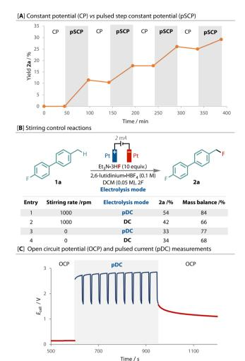
Fig. 4 A: Sequential direct and pulsed potential experiment showing how the yield of 2a only increases during the pulsed periods, but the loss of substrate 1a occurs under both regimes, albeit faster in pulsed. B: The effect of stirring on the direct and pulsed potential regimes; C: measurement of the open circuit potential before and after PP electrolysis.
