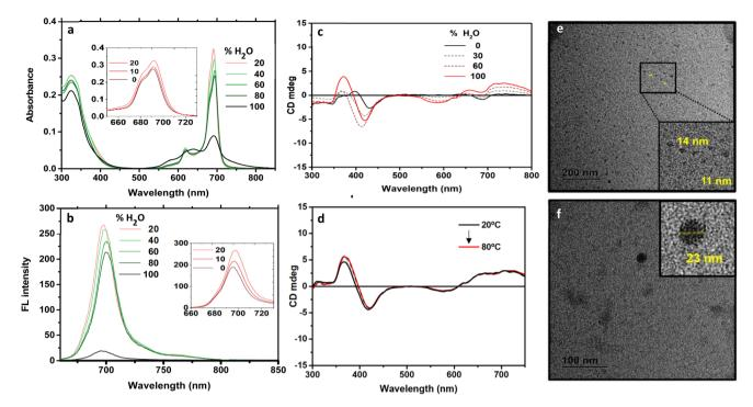
Fig. 3 (a) Absorption and (b) fluorescence spectral changes upon increasing the water ratio in solutions of 1 (5  $\times$  10<sup>-6</sup> M) in DMSO: water mixtures (Aexcitation = 650 nm). CD spectra of 1 (c) in DMSO and water at 20 °C and (d) on heating the solution from 20 °C to 80 °C at 1 °C min<sup>-1</sup> ([1] = 15 ×  $10^{-5}$  M) for temperature stability studies in pure water. (e) and (f) TEM images of 1 prepared using a water solution in ([1] =  $15 \times 10^{-5}$  M).
