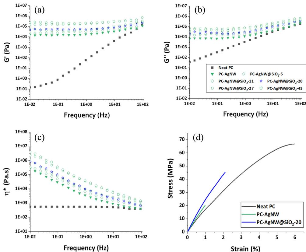
Fig. 4 (a)–(c) Rheological and (d) tensile properties of neat PC, PC-AgNW and PC-AgNW@SiO<sub>2</sub> nanocomposites: variations of (a) storage modulus, (b) loss modulus and (c) complex viscosity as a function of frequency at 250 °C; (d) averaged stress–strain curves of neat PC, PC-AgNW and PC-AgNW@SiO<sub>2</sub>-20 nanocomposites.
