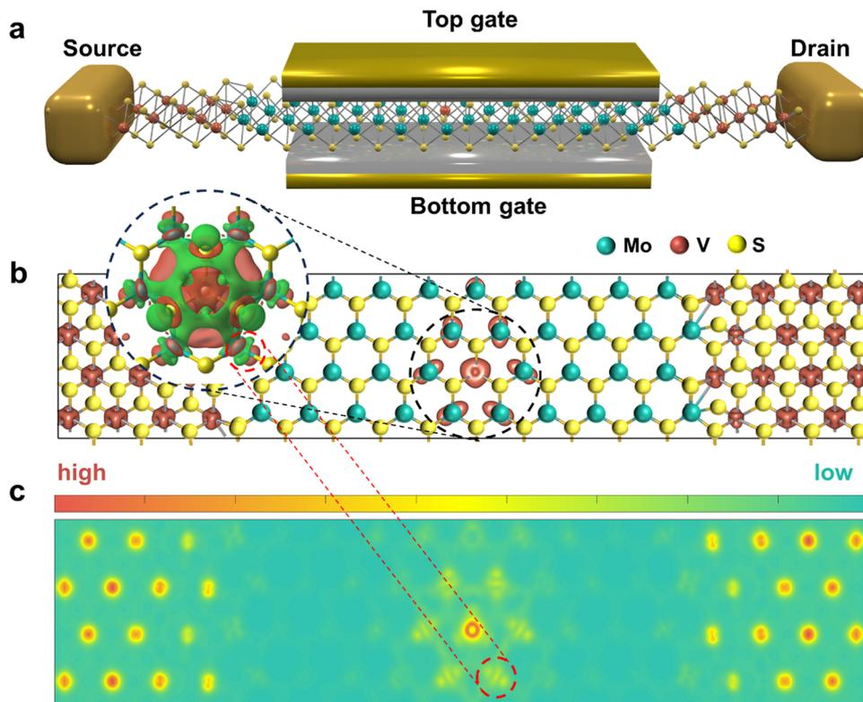
**Fig. 2** Schematic diagram of a FET model with  $\text{VS}_2$  electrodes at both ends,  $\text{V-MoS}_2$  channel in the middle ( $L_{\text{ch}} = 3.0$  nm), and gate electrodes (EOT = 0.5 nm) on top and bottom (a). The real-space DOS at  $-0.2$  eV (b) and corresponding 2D plot (c) are shown with zero source-drain bias applied. The inset in (b) represents the differential charge density at the V-doped site.
