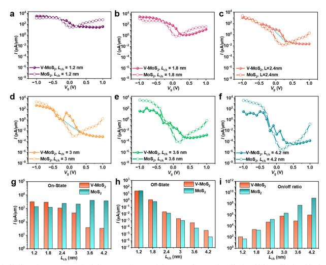
Fig. 3 (a)–(f) Transfer characteristics of  $MoS_2$  (hollow circles) and V- $MoS_2$  (solid spheres) at  $L_{ch}$  = 1.2 nm (a), 1.8 nm (b), 2.4 nm (c), 3.0 nm (d), 3.6 nm (e), and 4.2 nm (f), under a source bias of 0.2 V. Shown in (g-i) are the comparison of the on-state currents (g), off-state currents (h), and on/off ratios (i) between V- $MoS_2$  (orange) and  $MoS_2$  (cyan) at different  $L_{ch}$ .
