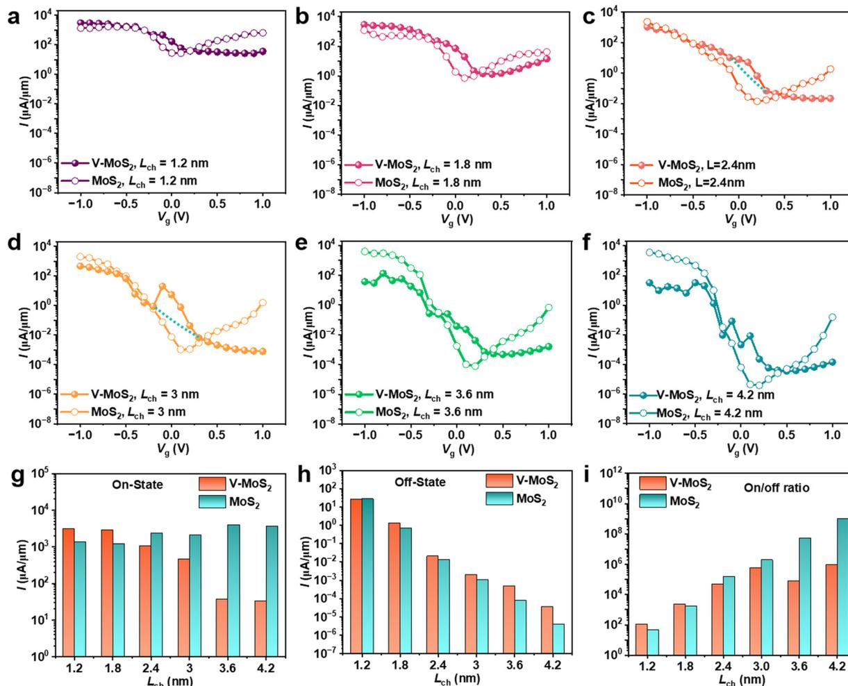
Fig. 3 (a)–(f) Transfer characteristics of MoS<sub>2</sub> (hollow circles) and V-MoS<sub>2</sub> (solid spheres) at  $L_{\text{ch}} = 1.2$  nm (a), 1.8 nm (b), 2.4 nm (c), 3.0 nm (d), 3.6 nm (e), and 4.2 nm (f), under a source bias of 0.2 V. Shown in (g–i) are the comparison of the on-state currents (g), off-state currents (h), and on/off ratios (i) between V-MoS<sub>2</sub> (orange) and MoS<sub>2</sub> (cyan) at different  $L_{\text{ch}}$ .
