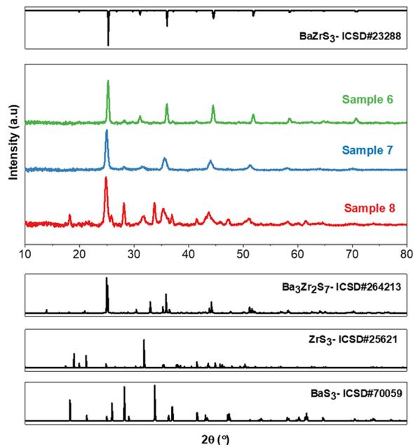
Fig. 2 XRD patterns of Ba–Zr–S films synthesized as described in Method 2 followed by 15 min sulfurization heat treatments at 575 °C in evacuated 5 mL ampules containing varying amounts of sulfur 0.31 mmol sulfur in Sample 6, 0.08 mmol in Sample 7 and 0.05 mmol in Sample 8. Fig. S3–S5 (ESI<sup>†</sup>) show Rietveld refinement for Samples 6, 7 and 8.
