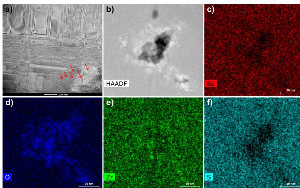
**Fig. 3** (a) TEM bright field image of a thin lamella prepared by FIB shows many planar defects and impurities in the grain. The red arrows point out examples of bright spots-indicating oxide impurities- in the image, one of which is analyzed using HAADF-STEM. (b) a HAADF-STEM image of a bright spot seen in the TEM bright field image. (c)–(f) EDX intensity maps of the HAADF image indicate the presence of zirconium oxide embedded in the BaZrS<sub>3</sub> grain.
