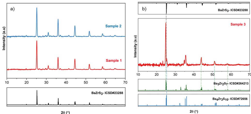
Fig. 1 XRD patterns of Ba–Zr–S films synthesized as described in Method 1 followed by 1 h sulfurization heat treatments at 575 °C in evacuated 5 mL ampules containing 0.03 mmol HfH<sub>2</sub> and (a) 0.45 mmol sulfur in Sample 1 and 0.30 mmol in Sample 2 or (b) 0.15 mmol sulfur in Sample 3. Fig. S2 (ESI<sup>†</sup>) shows Rietveld refinement for Samples 1 and 3.
