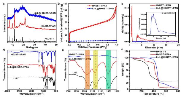
Fig. 3 Characterizations of HKUST-1/PAN and Li-IL@HKUST-1/PAN: (a) XRD, (b) BET nitrogen adsorption and desorption curve, (c) corresponding pore size distribution, (d) FT-IR, (e) locally amplified FT-IR, and (f) TGA curve.
