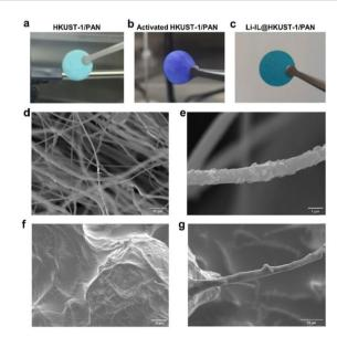
**Fig. 2** Image of open porositied HKUST-1/PAN: (a) before activation, (b) after activation, (c) after Li-IL loading, and SEMs of HKUST-1/PAN (d) and (e) and Li-IL@HKUST-1/PAN (f) and (g).
