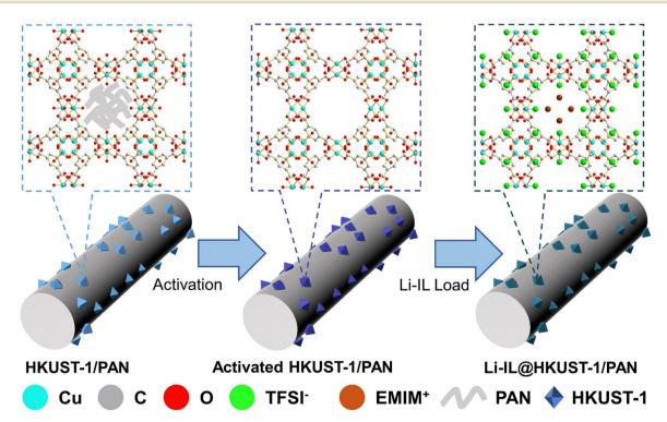
Fig. 1 Schematic of the efficient combination of HKUST-1, PAN and Li-IL into Li-IL@HKUST-1/PAN CSE.
