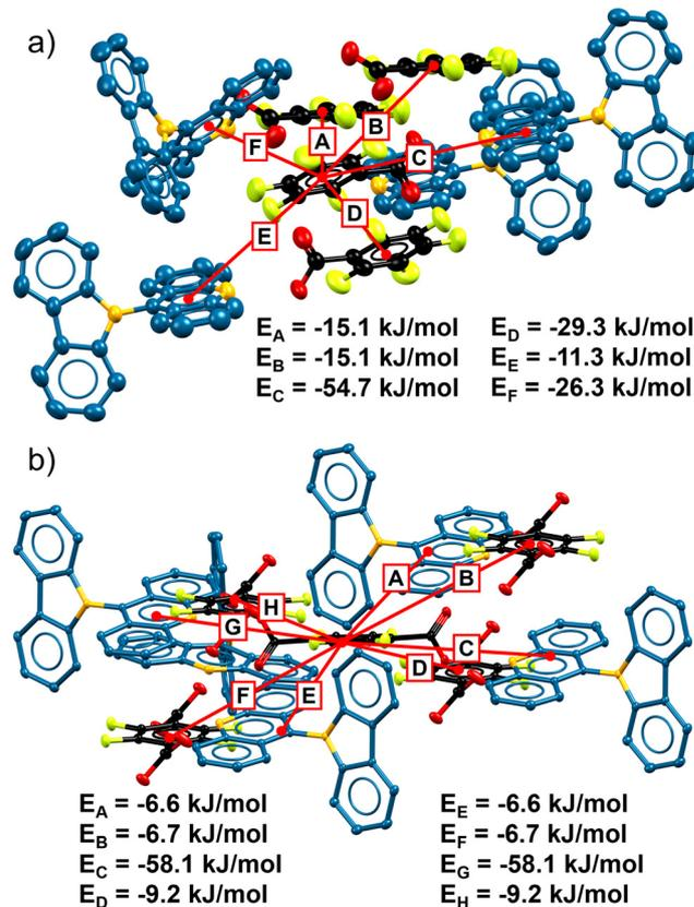
Fig. 5 Distribution of non-covalent interaction energies in (a) **AC-PFBA** and (b) **AC-TFTA**, obtained from calculations at the CE-B3LYP 6-31G(d,p) level of theory in CrystalExplorer 21.5.
