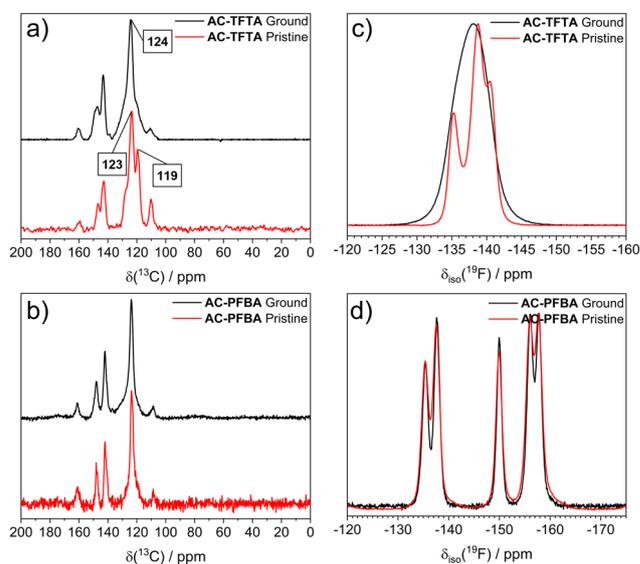
**Fig. 7** Characterization of pristine and ground powders of cocrystals through ssNMR.  $^{13}\text{C}$  MAS spectra with cross-polarization (125.8 MHz, Spin Rate = 20 kHz,  $d_1 = 20$  s) of (a) **AC-TFTA**, and (b) **AC-PFBA**  $^{19}\text{F}$  MAS spectra (470.6 MHz, Spin Rate = 20 kHz,  $d_1 = 10$  s) of (c) **AC-TFTA**, and (d) **AC-PFBA**. In these spectra, only the central signals are shown. For the full spectra, please visualize the ESI† file.
