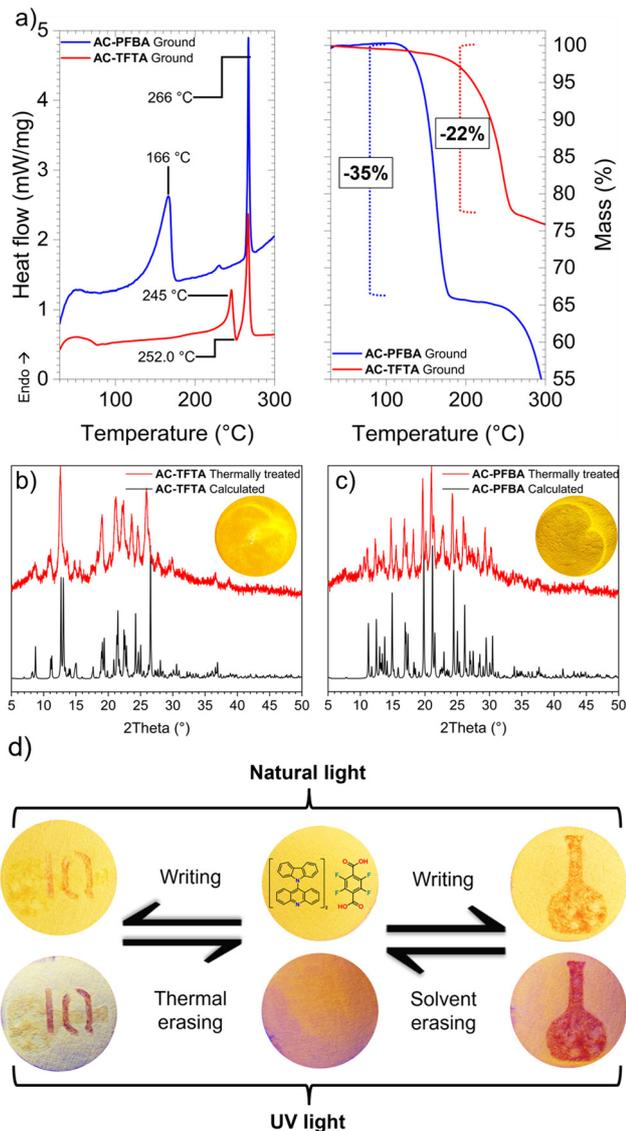
**Fig. 9** (a) DSC/TGA curves of ground powders; (b) and (c) PXRD profile of thermally treated powders of the cocrystals herein reported. As inset in each PXRD a picture shows the appearance of the powder after 10 minutes of heating on a hot plate at 80 °C under natural light; (d) drawing-erasing cycles with heat and DCM vapours of a filter paper with dispersion of AC-TFTA powders on the surface.
