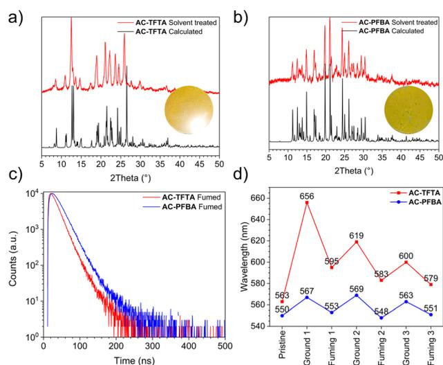
**Fig. 8** PXRD diffractograms of fumed samples compared against calculated PXRD form SC XRD for (a) AC-TFTA and (b) AC-PFBA. The appearance of the fumed solids is shown as insets in each diffractogram under natural light; (c) time-resolved fluorescence decay of the fumed samples and (d) relevant data from fatigue tests performed on the cocrystals. The regeneration of samples was carried out through the fuming of samples with DCM vapours.
