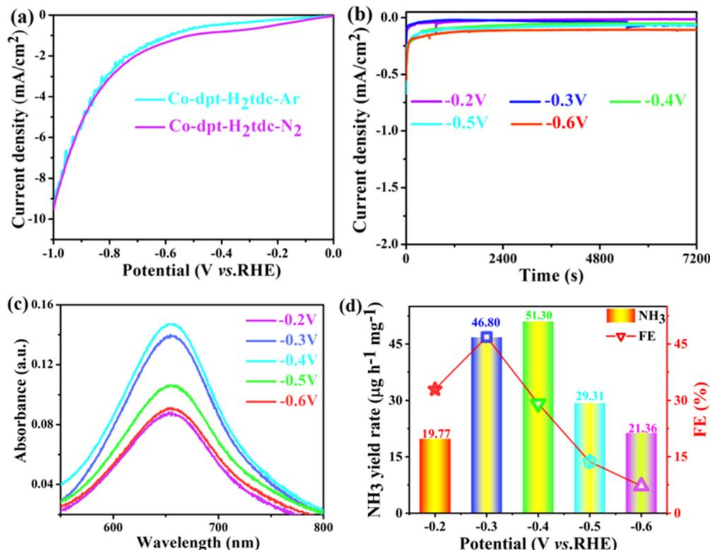
**Fig. 8** (a) Polarization curves of Co-dpt-H<sub>2</sub>tdc in N<sub>2</sub> and Ar-saturated 0.1 M Na<sub>2</sub>SO<sub>4</sub> electrolyte; (b) time-dependent current densities curves of Co-dpt-H<sub>2</sub>tdc at different potentials from -0.2 V to -0.6 V; (c) UV-vis spectra were estimated with the indophenol blue method at five given voltages for Co-dpt-H<sub>2</sub>tdc; and (d) NH<sub>3</sub> yield and FE of Co-dpt-H<sub>2</sub>tdc at different potentials from -0.2 V to -0.6 V.
