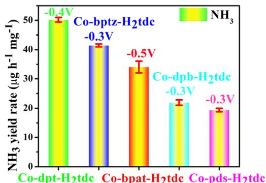
Fig. 11 NH<sub>3</sub> yield rate of five Co-MOF-based electrocatalysts based on similar ligands at their respective maximum potential.
