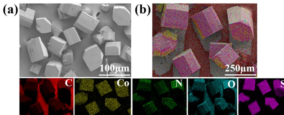
Fig. 6 (a) SEM and (b) EDS of Co-dpt-H<sub>2</sub>tdc.
