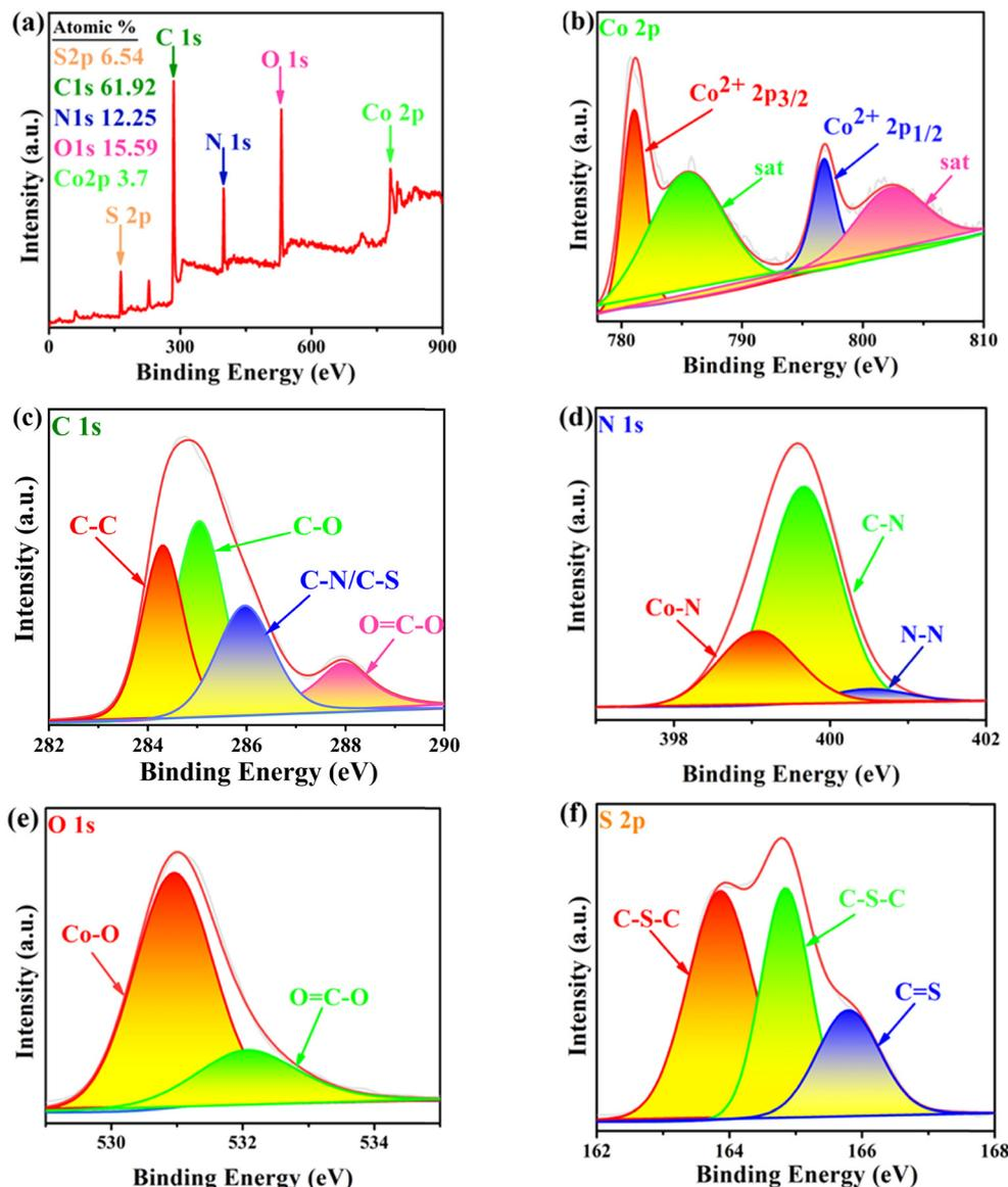
Fig. 7 (a) XPS full spectra of Co-dpt-H<sub>2</sub>tdc; (b) Co 2p; (c) C 1s; (d) N 1s; (e) O 1s; and (f) S 2p.
