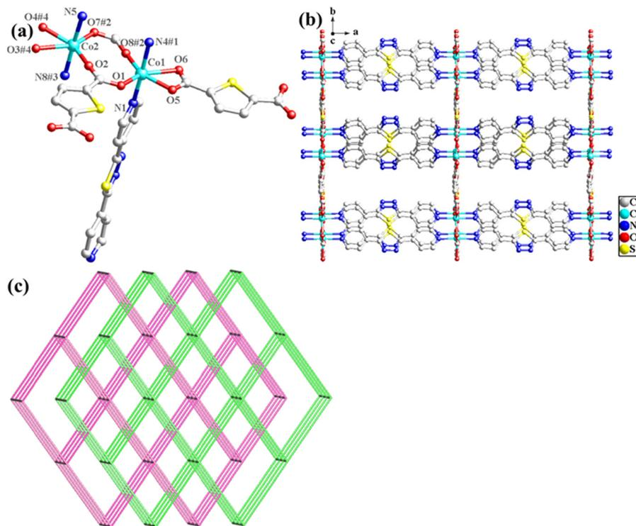
**Fig. 1** (a) Coordination environment of Co(II) ions of Co-dpt-H<sub>2</sub>tdc, symmetry code: #1 = 1 + x, y, z; #2 = x, 1/2 - y, -1/2 + z; #3 = -1 + x, y, z; #4 = x, 3/2 - y, -1/2 + z; (b) three-dimensional structure diagram of Co-dpt-H<sub>2</sub>tdc; and (c) 2-fold interpenetrating **pcu** topology of Co-dpt-H<sub>2</sub>tdc.
