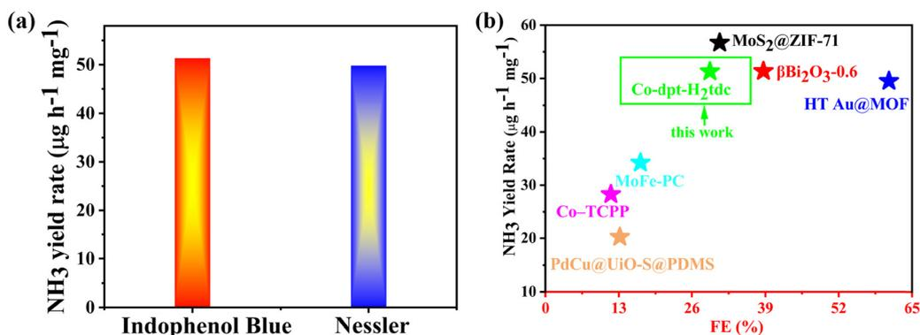
**Fig. 10** (a) Comparison of the NH<sub>3</sub> yield for NH<sub>3</sub> of Co-dpt-H<sub>2</sub>tdc at  $-0.4$  V measured by Nessler's reagent spectrophotometry and indophenol blue spectrophotometry; (b) comparison of eNRR performances with those of some reported electrocatalysts.
