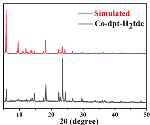
Fig. 5 PXRD pattern of synthesized Co-dpt-H<sub>2</sub>tdc and standard spectra simulated using single crystal data.
