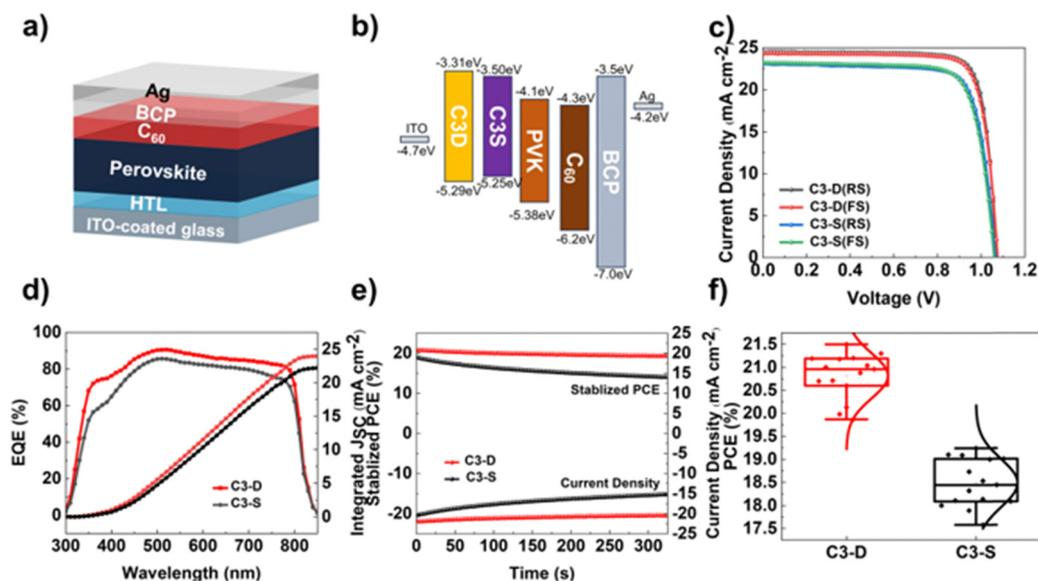
Fig. 5 (a) Device structure diagram; (b) diagram of the energy levels; (c) *J*–*V* curves measured by forward and reverse scans of the champion devices; (d) EQE spectrum and integrated short-circuit current density; (e) stability output curves at the maximum power point of the devices; and (f) the PCE statistics of devices.
