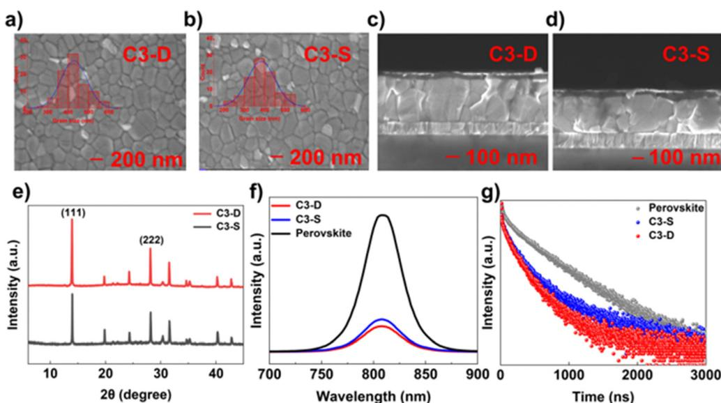
Fig. 4 SEM of perovskite film deposited on (a) C3-D, and (b) C3-S. Cross-sectional SEM of PSCs fabricated on (c) C3-D, and (d) C3-S. (e) XRD patterns of perovskite films deposited on C3-D and C3-S. (f) PL spectra and (g) TRPL spectra of perovskite films.
