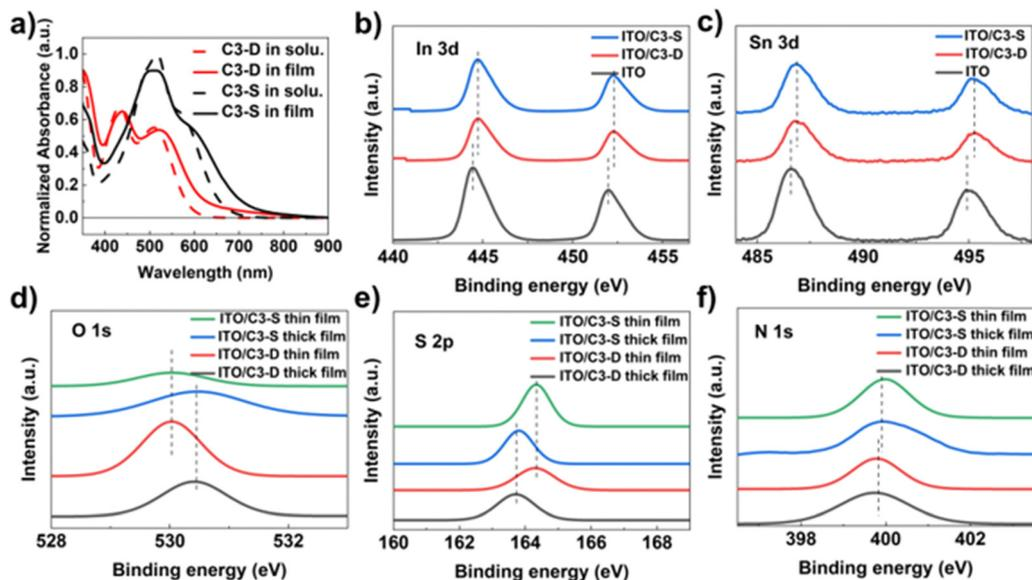
Fig. 2 (a) UV-vis absorption spectra of C3-D and C3-S; XPS spectra of (b) In 3d, (c) Sn 3d, (d) O 1s, (e) S2p, and (f) N1s for C3-D, C3-S deposited on ITO and bare ITO.
