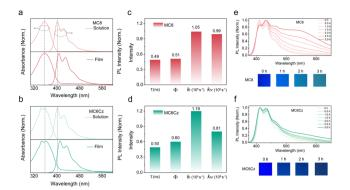
Fig. 1 Optical property of MC8 and MC6Cz. Absorption and PL spectra of MC8 (a) and MC6Cz (b) in solutions and spin-coated films from toluene solutions. Fluorescence lifetime, photoluminescence quantum yield, radiative and non-radiative transition rates ( $k_r = \Phi/\tau$ ,  $k_{nr} = 1/\tau - k_r$ ) of **MC8** (c) and MC6Cz (d) spin-coated films. PL spectra of MC8 (e) and MC6Cz (f) aged films. The aged films were prepared by continuous irradiation of spin-coated films under a 365 nm UV lamp.
