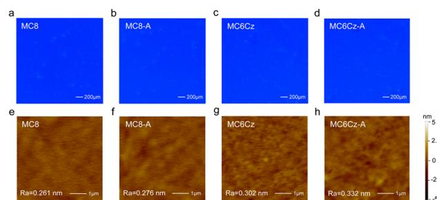
Fig. 3 Fluorescence microscopy (FLM) and atomic force microscopy (AFM) images of pristine films of **MC8** (a) and (e), **MC6Cz** (c) and (g), annealed films of **MC8** (b) and (f), **MC6Cz** (d) and (h). The annealed film was prepared after thermal treatments at 120 °C in a nitrogen atmosphere for 15 min.
