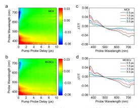
Fig. 2 Transient absorption (TA) analysis of MC8 and MC6Cz films. TA contour plots of MC8 (a) and MC6Cz (b). (c) and (d)  $\Delta T/T$  spectra of MC8 and MC6Cz films from 0.5 to 5.0 ps pump-probe delay.
