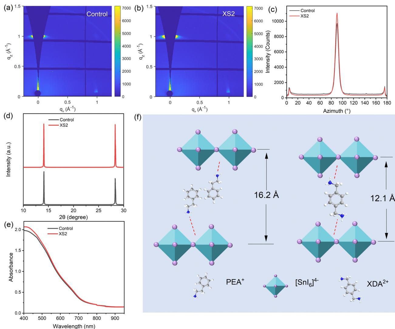
**Fig. 1** Characterization of the perovskite crystal structures. (a) GIWAXS patterns of control films and (b) XS2 films with an incident angle of  $0.5^\circ$ . (c) GIWAXS intensity integrated azimuth at  $q = 1 \text{ \AA}^{-1}$ . (d) XRD patterns and (e) Abs spectra of control and XS2 films. (f) Schematic of interaction between  $[\text{SnI}_6]^{4-}$  and PEA (left) or XDA (right).
