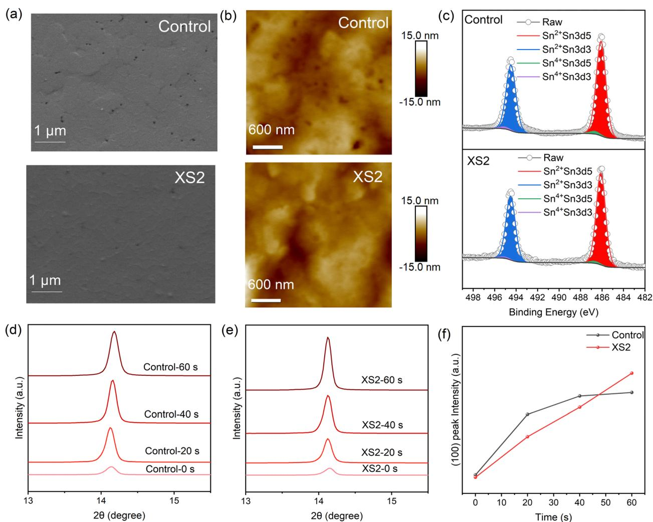
**Fig. 2** Characterization of perovskite films. (a) SEM pictures of control and XS2 films. (b) AFM pictures of control and XS2 perovskite films. (c) The XPS result of the control and XS2 films. (d) The XRD patterns of the control films and XS2 films (e) based on different annealing times. (f) The (100) plane diffraction intensity of the control and XS2 perovskite thin films based on different annealing times.
