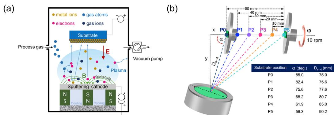
Fig. 3 (a) Schematic representation illustrating the principle of magnetron sputtering technology,<sup>55</sup> adapted with permission from ref. 55, copyright 2020 by Elsevier Ltd and Techna Group S.r.l. (b) Diagram of the magnetron sputtering with glancing angle deposition (MS-GLAD) technique,<sup>56</sup> indicating that the substrate can be adjusted from positions P0 to P5, adapted with permission from ref. 56, copyright 2021 by Elsevier Ltd and Techna Group S.r.l.
