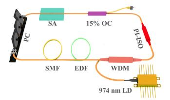
Fig. 5 Schematic diagram of the mode-lcoked erbium-doped fiber laser.
