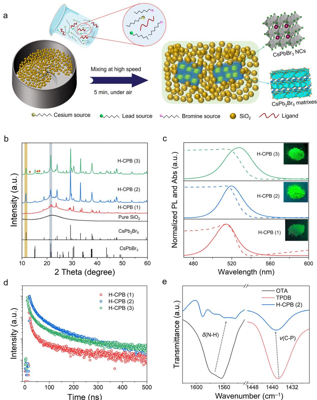
**Fig. 1** Preparation and performance of H-CPB composites. (a) Schematic illustration of the fabrication process for H-CPB composites. (b) Powder XRD patterns of pure SiO<sub>2</sub> and H-CPB composites. (c) UV-vis absorption and PL spectra of H-CPB composites. Inset: Photographs of H-CPB composites under the irradiation of UV light (365 nm). (d) PL decay kinetics for H-CPB composites. (e) FTIR spectra of OTA, TPDB, and the H-CPB (2).
