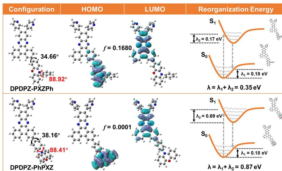
**Fig. 2** Molecular configurations and frontier molecular orbital distributions (FMOs) of DPDPZ-PXZPh and DPDPZ-PhPXZ, and their reorganization energies ( $\lambda_{ex}$ ) between the  $S_0$  and  $S_1$  states.
