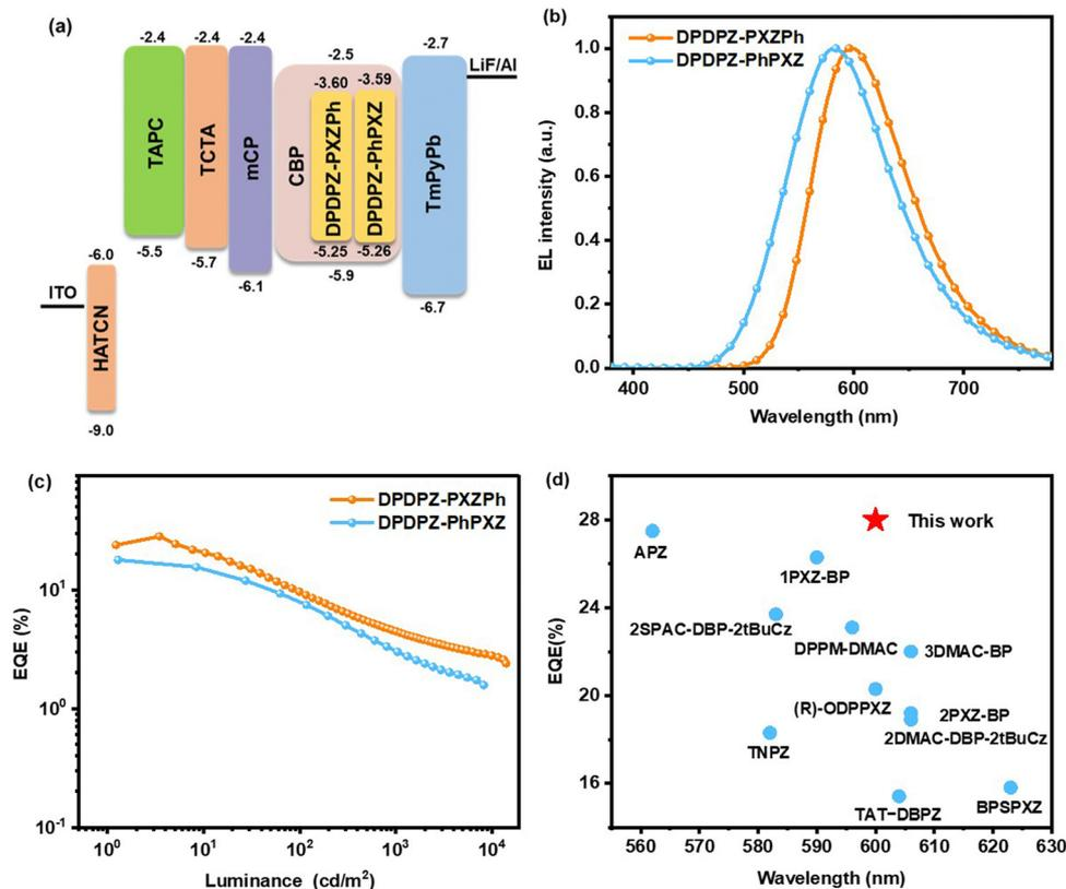
Fig. 5 EL performances of DPDPZ-PXZPh- and DPDPZ-PhPXZ-based OLEDs. (a) The configuration of OLED devices. (b) EL spectra at the optimized doping concentrations. (c) EQE versus luminance curves. (d) EQE summary of TADF materials based on the dibenzo[*a,c*]phenazine backbone with EL spectral peaks in the range of 560–630 nm (see Table S2 for details, ESI<sup>†</sup>).
